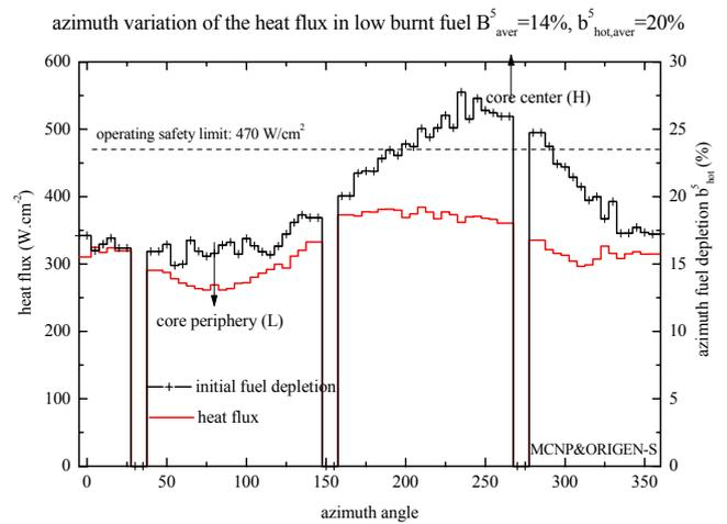
*Detailed heat flux distributions in the standard BR2 fuel elements in function of the BR2 configuration, the burn-up in the fuel plates and the azimuthal orientation of the concerned fuel element.*
