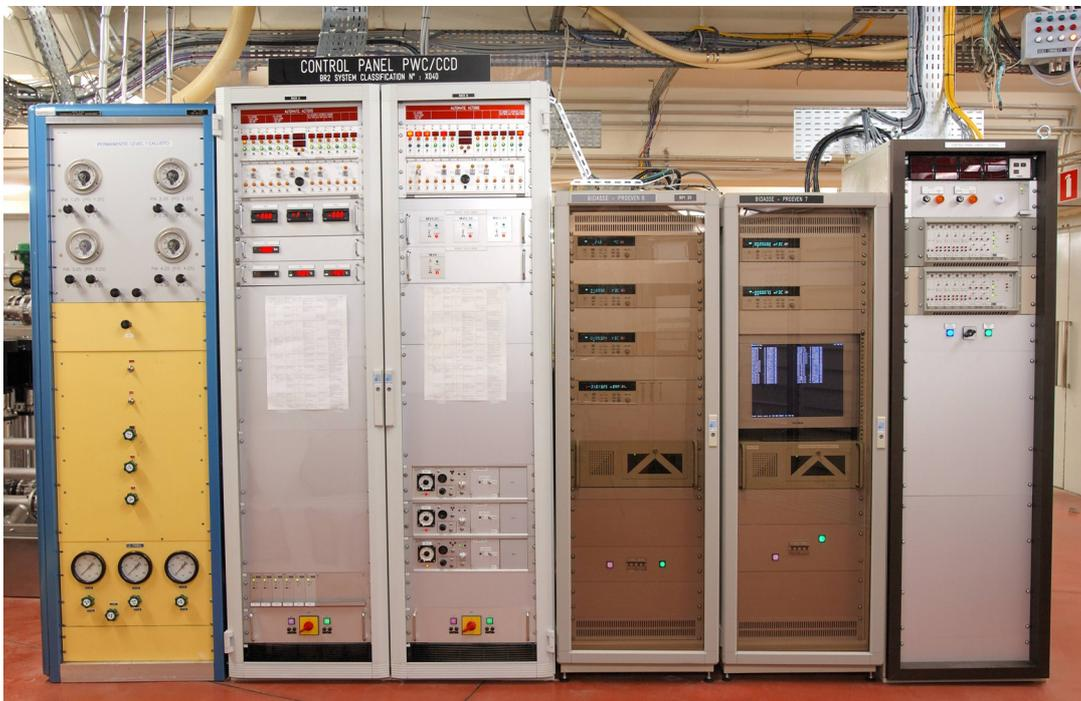
*Typical control and acquisition installation for an irradiation experiment: on left side the main control panel of the PWC/CCD irradiation device and on the right side the BIDASSE front end cabinets.*
