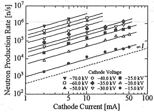
Fig. 4 Neutron production rate vs. cathode current at constant voltages (basic setup)
