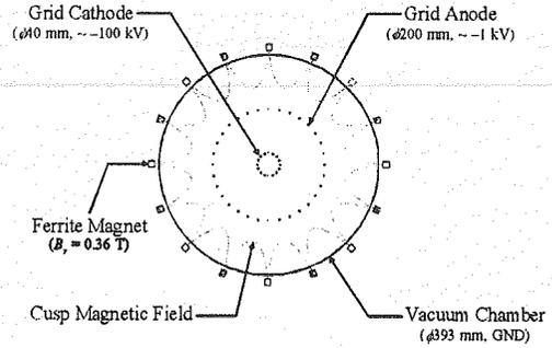
Fig. 2 Cross section of the cylindrical IECF device
