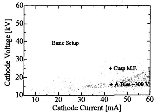
Fig. 10 Experimental condition of stable dc discharge
