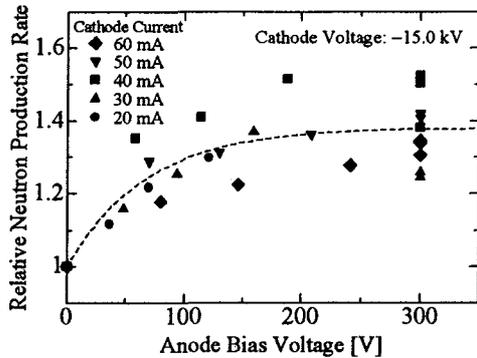
Fig. 8 Relative neutron production rate vs. anode bias voltage at a cathode voltage of  $-15.0$  kV
