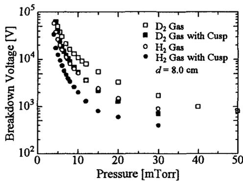
Fig. 6 Breakdown voltage vs. gas pressure
