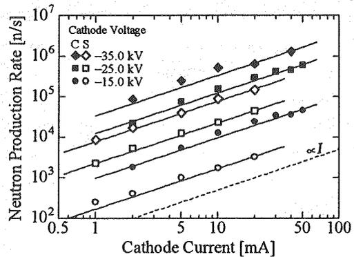
Fig. 5 Comparison of neutron production rate between the basic setup (C) and the conventional spherical device (S)
