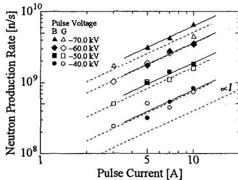
Fig. 11 Neutron production rate vs. pulse current (B: anode bias voltage of  $-1.0$  kV, G: anode grounded)
