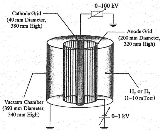
Fig. 1 Schematic of the cylindrical IECF device
