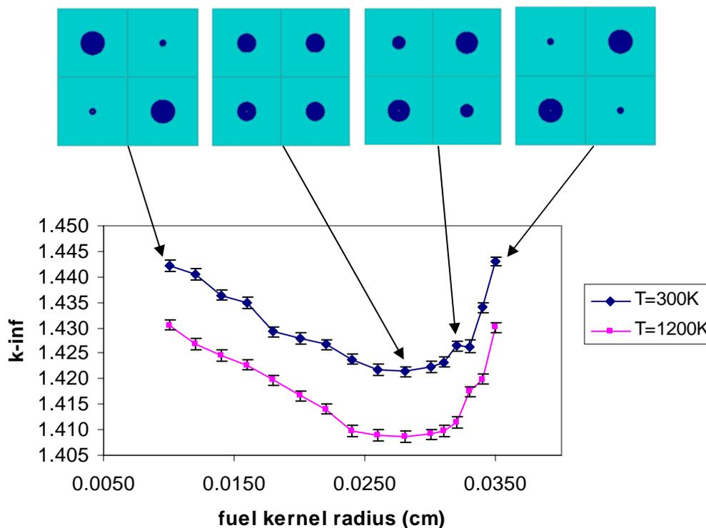
Figure 2: K-infinity as a function of fuel kernel radius at two different temperatures and fuel enrichment of 8 %. Above the chart there are views of the MCNP model of the cubic unit cell.
