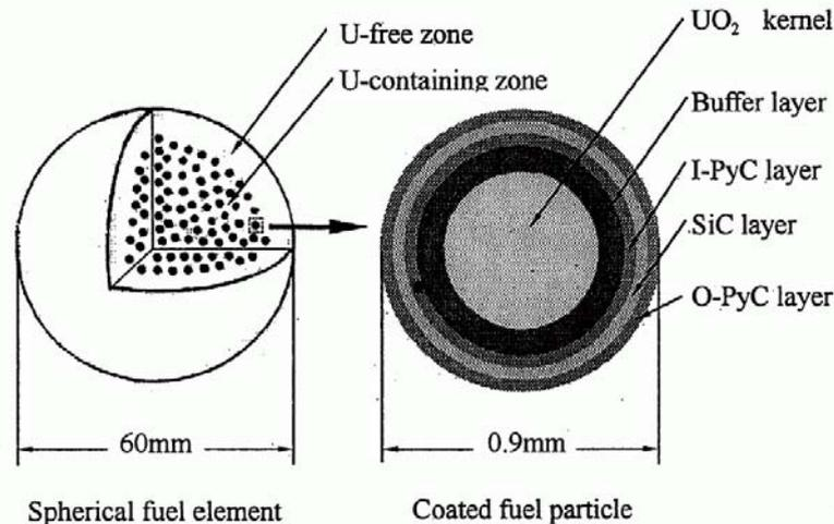
Figure 1: PBR spherical fuel element and coated fuel particle [1]
