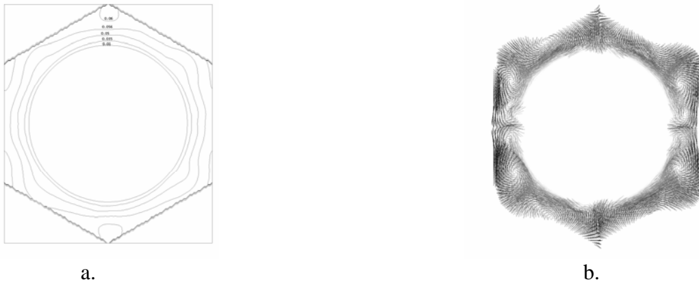
Fig. 6 Contours of the mean axial velocity (a) and the projection of the mean lateral velocities (b) to a cross section.
