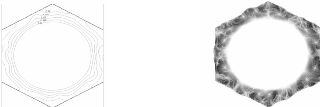
Fig. 3 Contours of the mean axial velocity (left) and the projection of the mean lateral velocities to a cross section.
