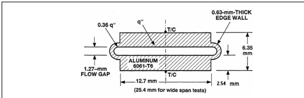
Figure 2: cross section of the test section and the cooling channel [4]
