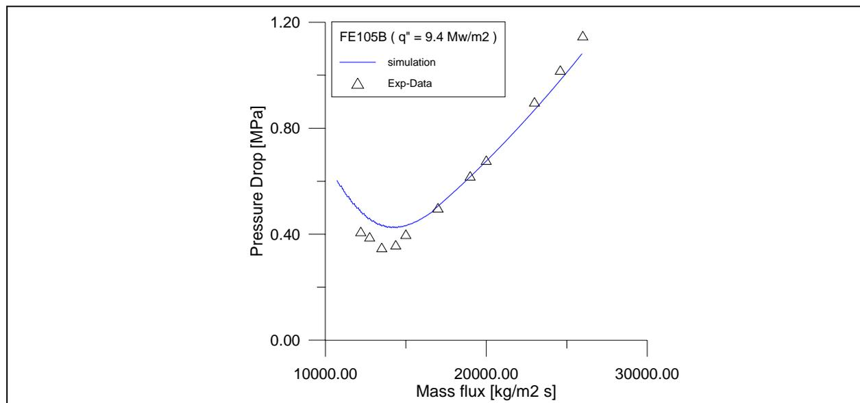
Figure 7: Pressure drop for heat flux of 9.4 MW/m<sup>2</sup>
