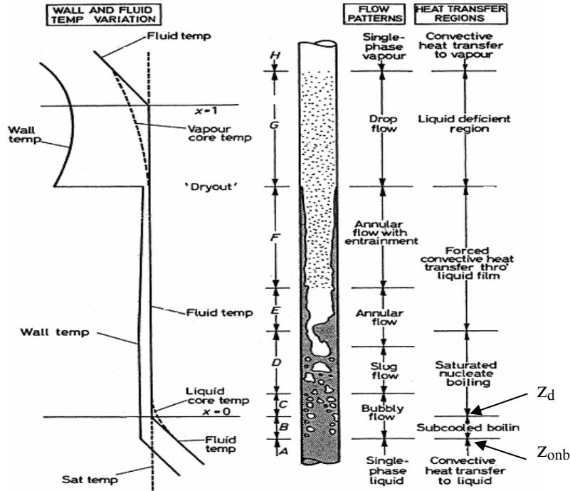
Figure 1: Patterns encountered in a vertical upward flow in a heated channel [5]
