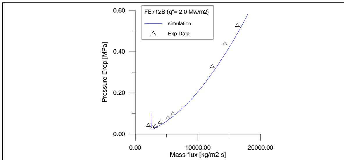
Figure 4: Pressure drop for heat flux of 2.0 MW/m<sup>2</sup>
