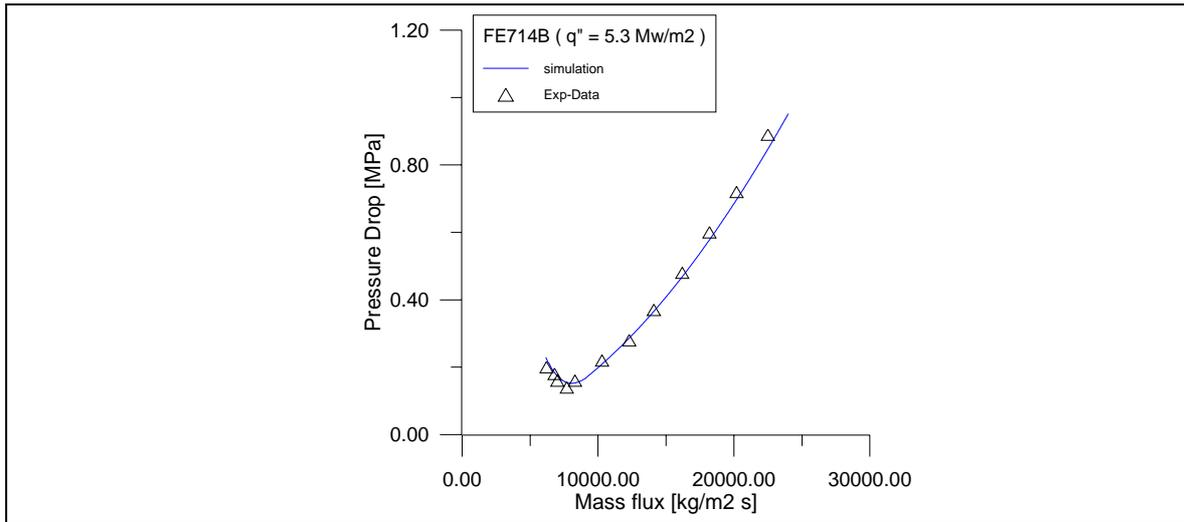
Figure 5: Pressure drop for heat flux of 5.3 MW/m<sup>2</sup>
