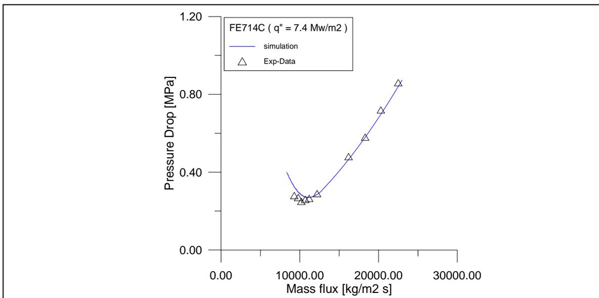
Figure 6: Pressure drop for heat flux of 7.4 MW/m<sup>2</sup>
