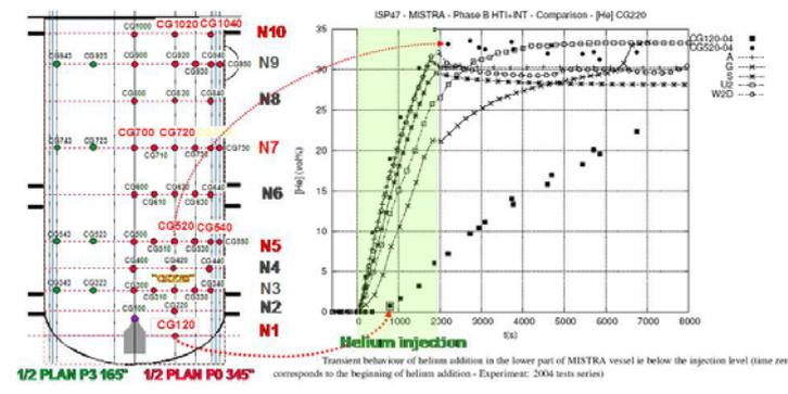
Figure 10 : Transient behaviour of helium addition in the lower part of MISTRA vessel ie below the injection level (time zero corresponds to the beginning of helium addition - Experiment: 2004 tests series)
