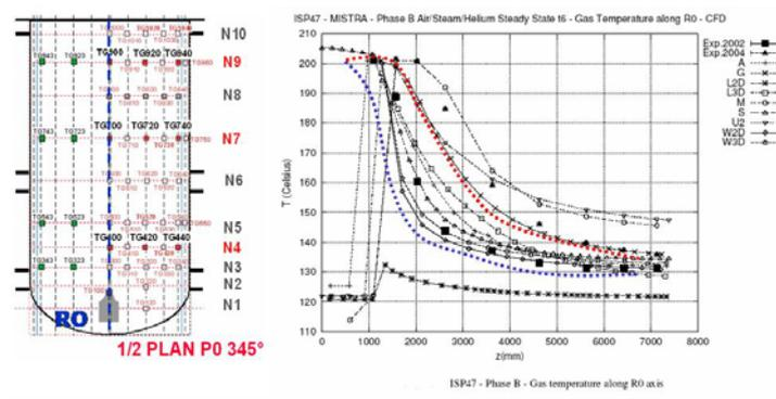
Figure 9 : ISP47 - Phase B - Gas temperature along R0 axis
