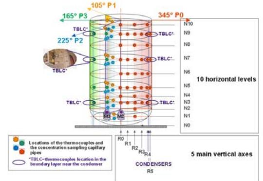
Figure 4: Sketch of MISTRA's instrumental mesh grid for free volume configuration
