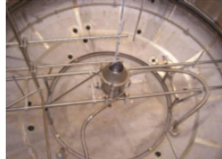
Figure 3 : View of 200mm injection nozzle, here positioned at the centre (ie. for ISP-47 test)
