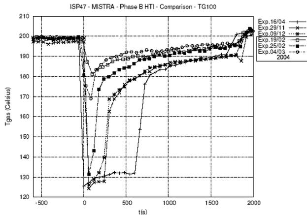
Figure 5: ISP47: injection temperature of the gaseous mixture (Steam and Helium) during the transient addition of helium (2002 tests series: 16/04, 29/11 and 09/12 - 2004 tests series 19/02, 25/02 and 04/03) [8]
