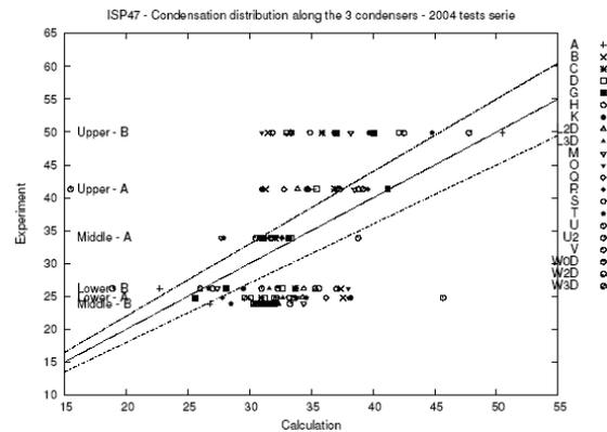
Figure 8 : Condensation distribution for the two steady-states A and B - 2004 tests series (lines correspond to 10% deviation)
