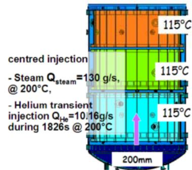
Figure 6: Sketch of MISTRA specification boundary conditions for ISP47 test.
