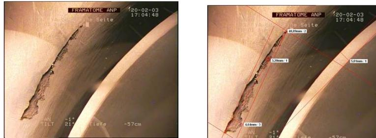
Figure 5: Image analysis: sizing of discontinuities
