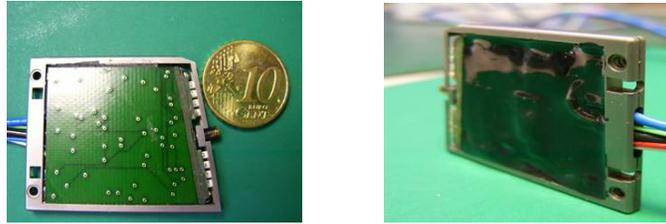
Figure 3: 2.6-mm camera for steam generator inspections (prototype)
