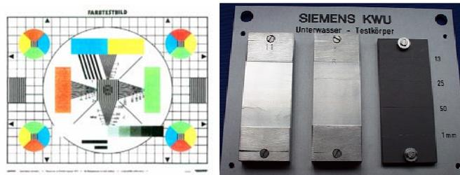
Figure 4: Test patterns and reference blocks for camera calibration
