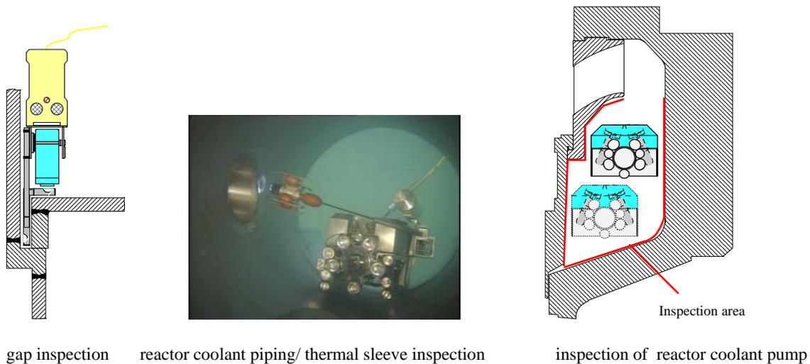
Figure 8: Examples of inspections using SUSI
