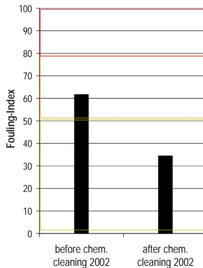
Figure 7: Example: Overall fouling index before and after chemical cleaning
