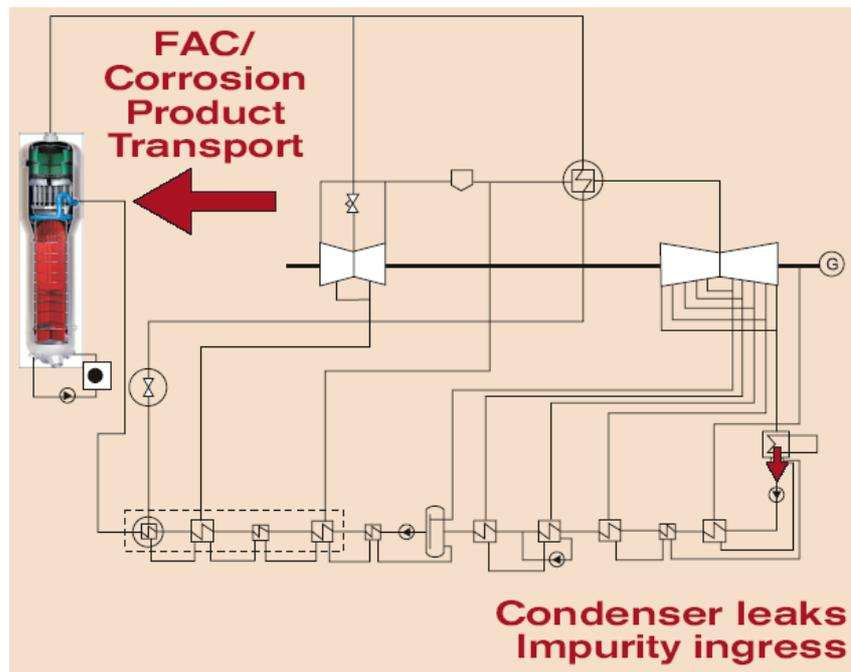
Figure 1: Impurity ingress into the steam generator
