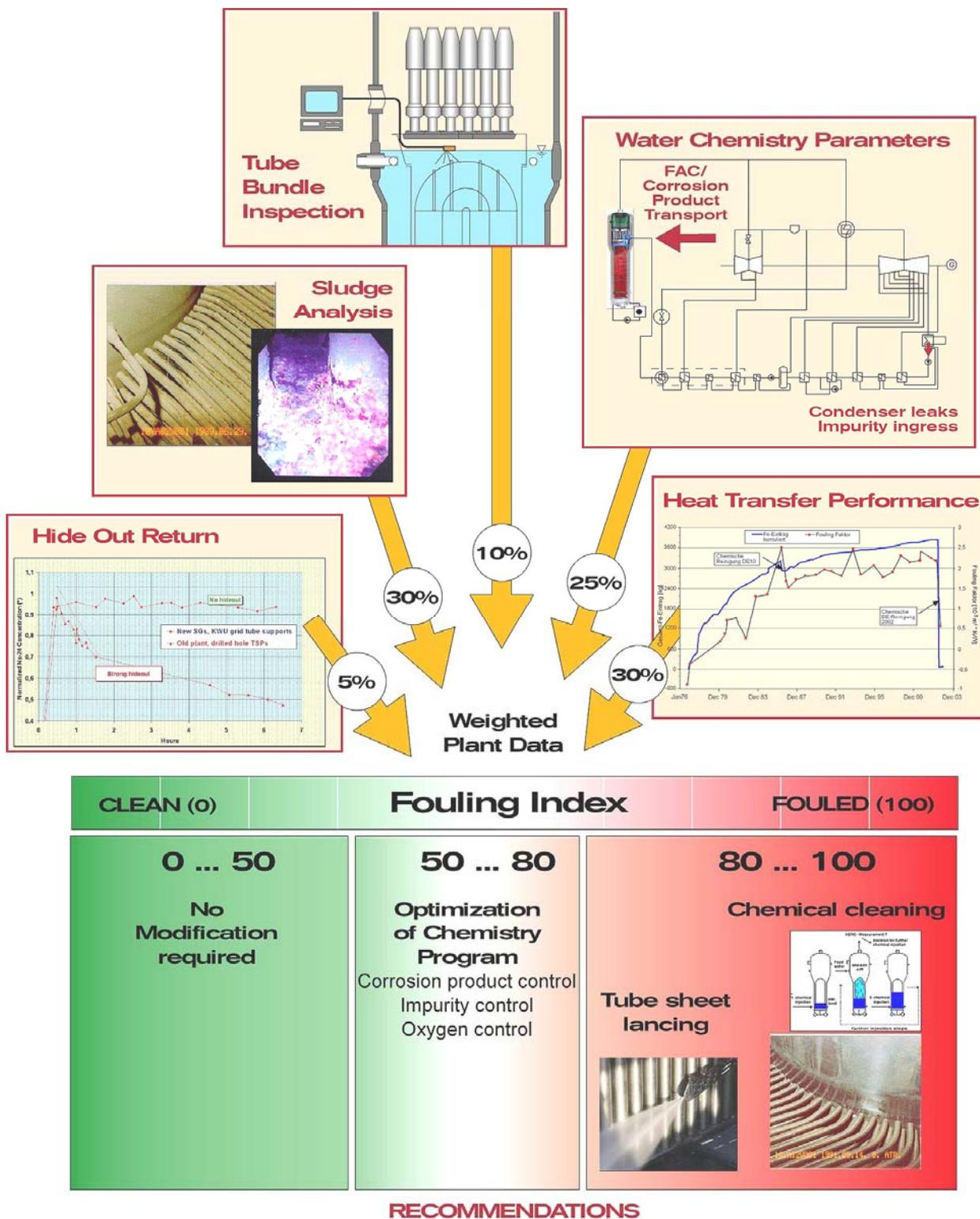
Figure 8: Summary: fouling index and derived cleaning recommendations
