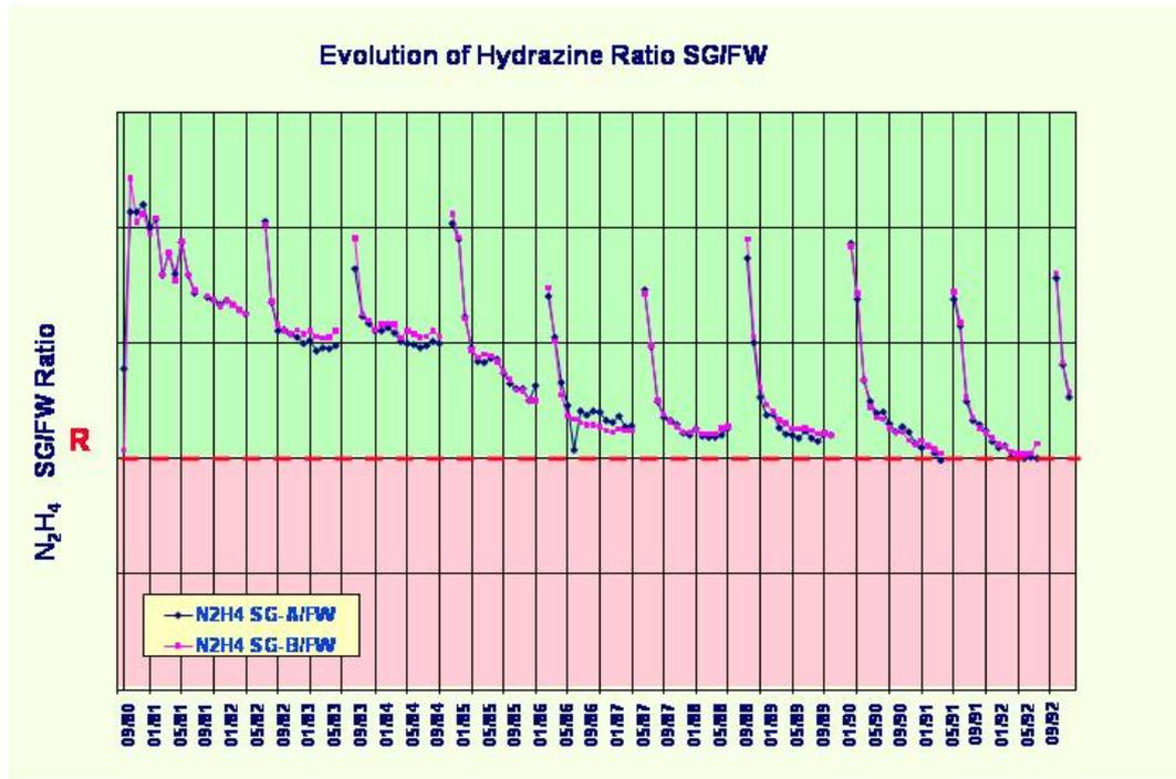
Figure 4: Typical evolution of hydrazine concentration ratio SG/FW in a PWR
