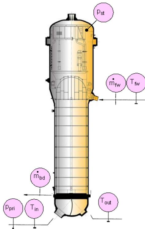
Figure 2: Operational data to be recorded for thermal performance monitoring
