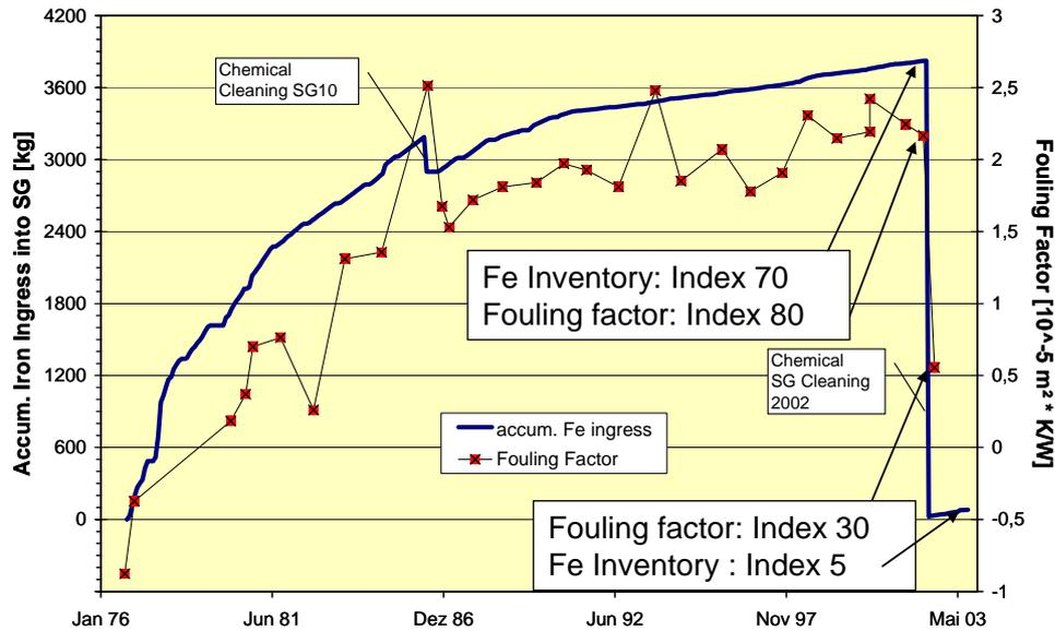
Figure 3: Fouling factor evolution vs. operating time correlated with Fe inventory. Effect of chemical cleaning. Index of fouling indicators before and after chemical cleaning
