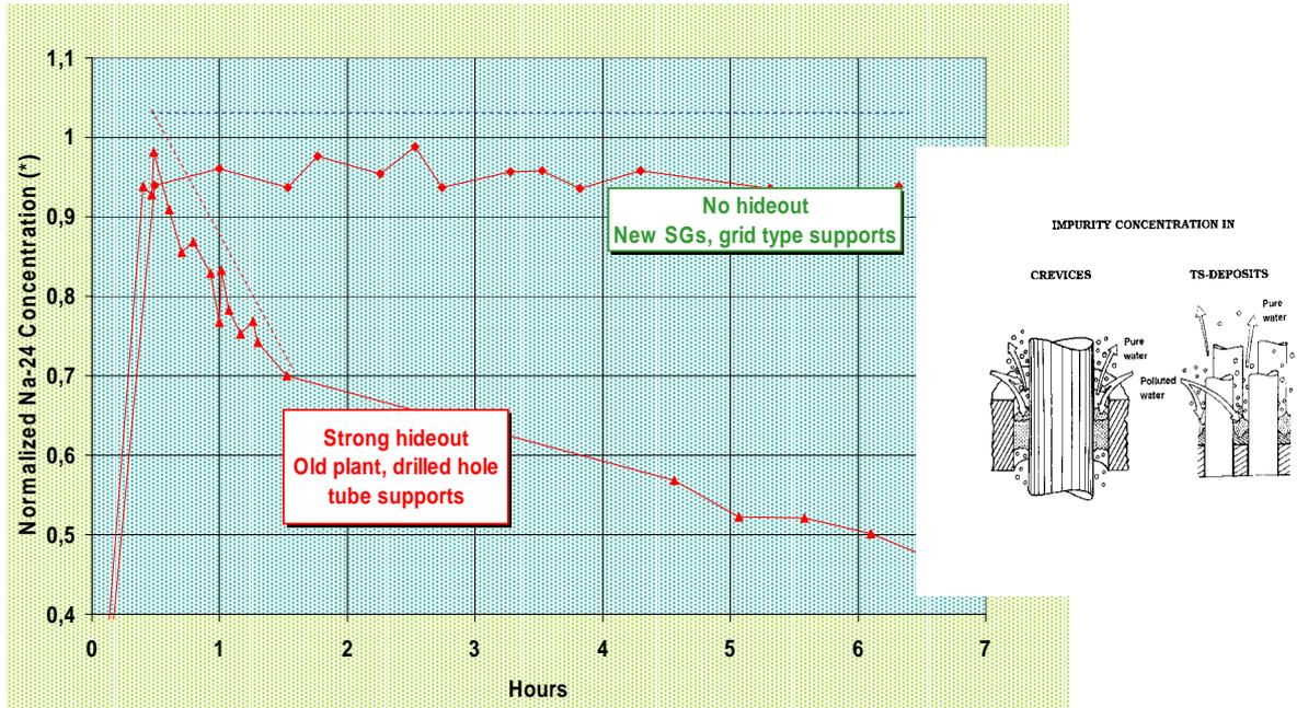
Figure 5: SGs with significant and negligible hide-out behavior
