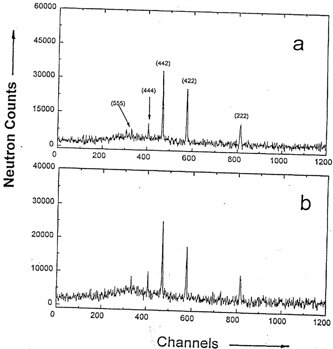
Fig.1. Measured diffraction patterns of copper; a) stress free sample. b) at welding point.
