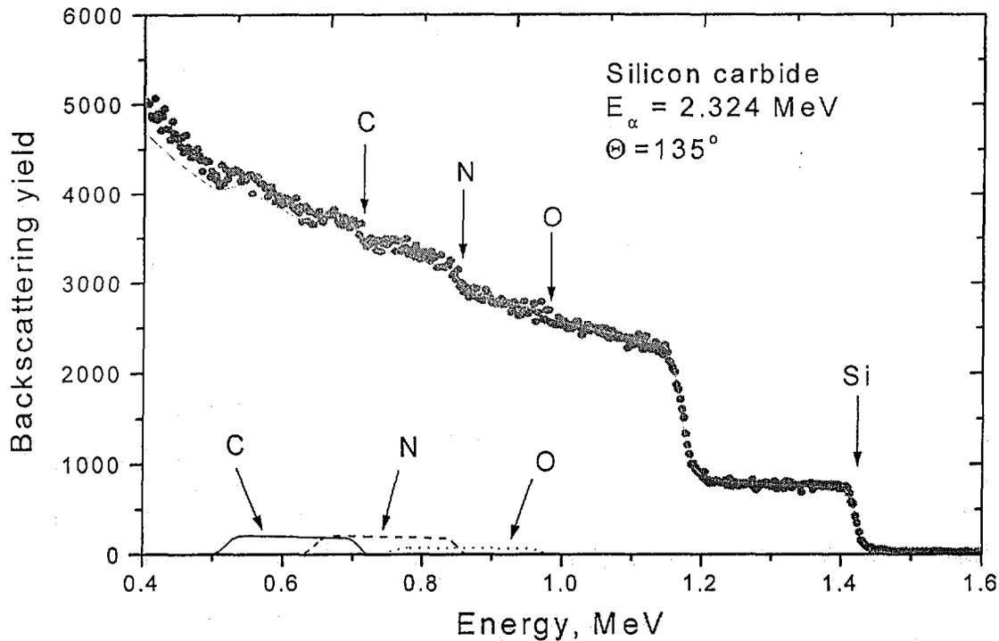
Fig. 5. Experimental and simulated spectra for SiC sample.
