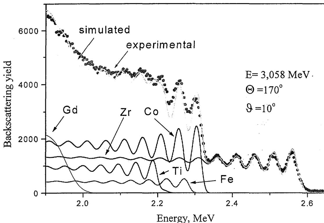
Fig.2. Spectra of 3.058 MeV  $^4\text{He}$  ions backscattered at TiZr/FeCo multilayer structures with period of 15.3nm. Partial spectra for heavy elements are shown.
