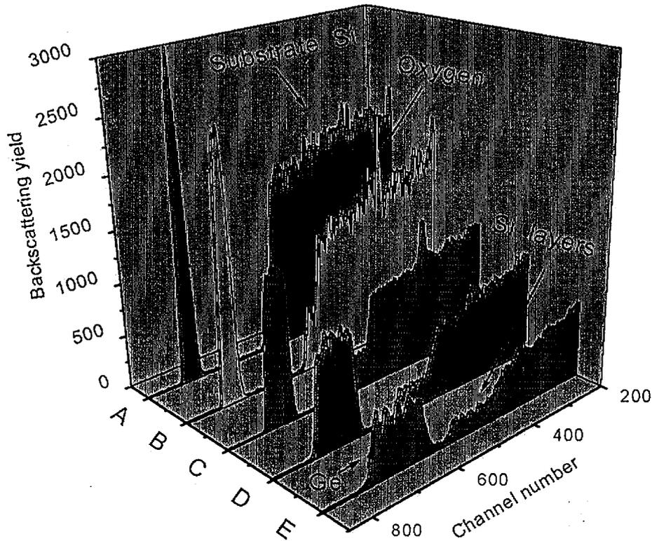
Fig. 1. spectra of 3.112 MeV  $^4\text{He}$  ions scattered at  $170^\circ$  by the Si/Ge multilayer structure. The incidence angle  $\varphi = 6^\circ - E$ ,  $\varphi = 10^\circ - D$ ,  $\varphi = 20^\circ - C$ ,  $\varphi = 40^\circ - B$ ,  $\varphi = 60^\circ - A$ .
