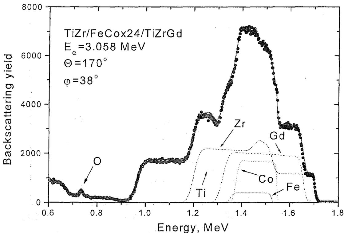
*Fig.3. Experimental and simulated spectra for the incident angle of  $38^\circ$  obtained at TiZr/FeCo multilayer structure.*
