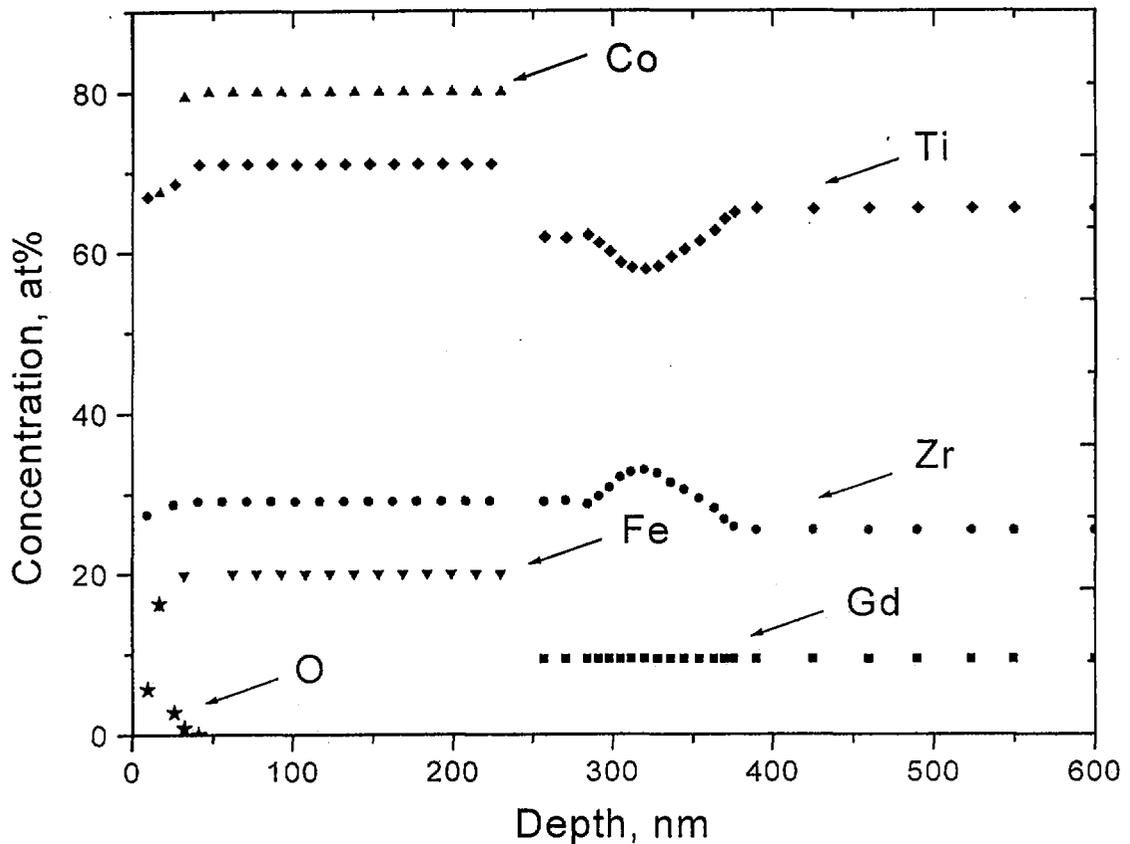
Fig.4. Element depth distribution for TiZr/FeCo multilayer structure derived from RBS and NRA experiments.
