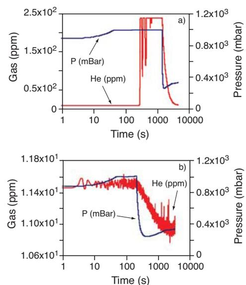
Fig. 3.30 - Helium migration from VV to vault (hot walls, 110°C)
