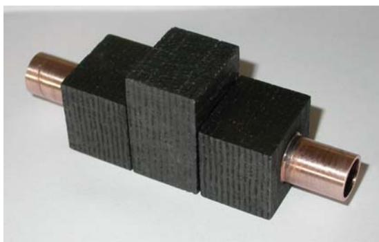
Fig. 3.1 - Monoblock mockup with three CFC tiles after HRP manufacturing
