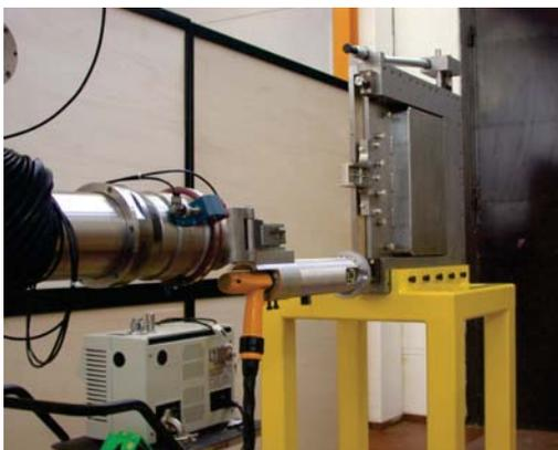
Fig. 3.28 - IFMIF lithium target back-plate reliability test
