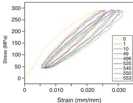
Fig. 3.23 - Bending cycles under high peak stress at RT (290 MPa)
