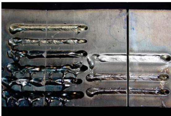
Fig. 3.13 - Melt runs performed on AISI stainless steel to set up the welding characteristics of the EBW machine at Ansaldo Superconduttori
