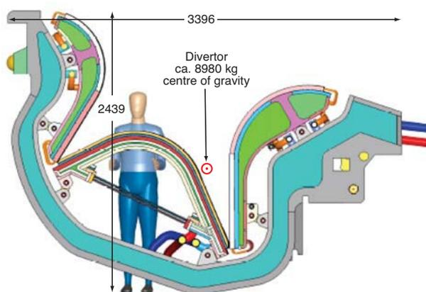
Fig. 3.17 - Model of the second new cassette prototype
