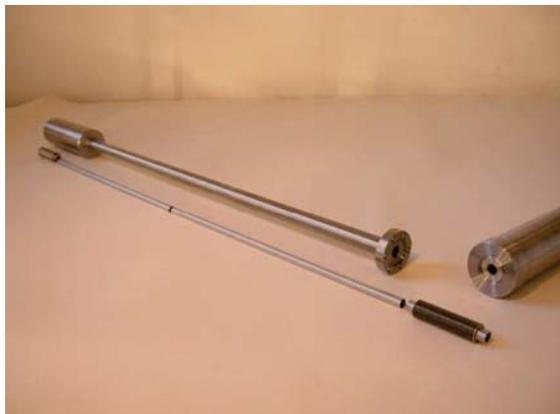
Fig. 3.11 - Main parts of the PERMCAT reactor: palladium tube, metal bellows and reactor shell
