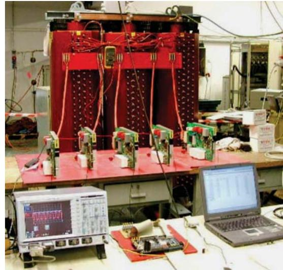
Fig. 3.14 - Testing of first ITER CDP gyrotron body power-supply modules with the related transformer
