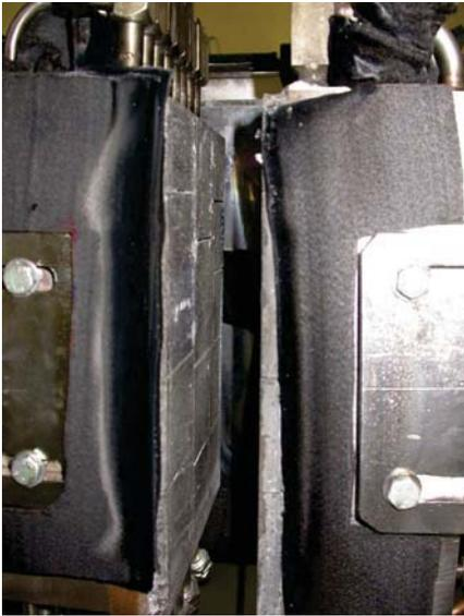
Fig. 3.4 - EDA III mockup assembly after 8244 fatigue cycles – lateral view without resistor
