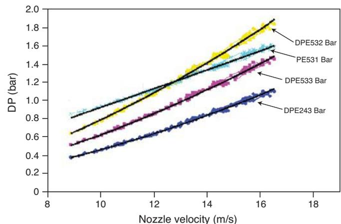
Fig. 3.27 - Hydraulic characteristics of the flow straightener and orificed plates (back-plate curvature 250 mm,  $T = 55^{\circ}\text{C}$ )
