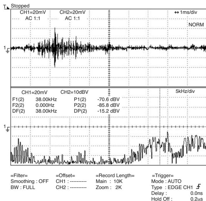
Fig. 3.26 - Cavitation at EMP inlet (nozzle velocity 13.3 m/s and argon pressure 0.065 MPa)
