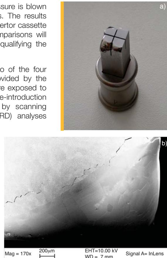
Fig. 3.3 - a) Tungsten sample after exposure in the FTU scrape-off layer; b) SEM image of the molten zone
