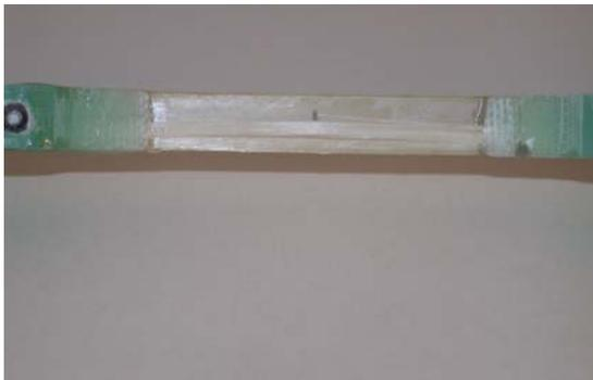
Fig. 3.12 - Collapsed sample of fibreglass
