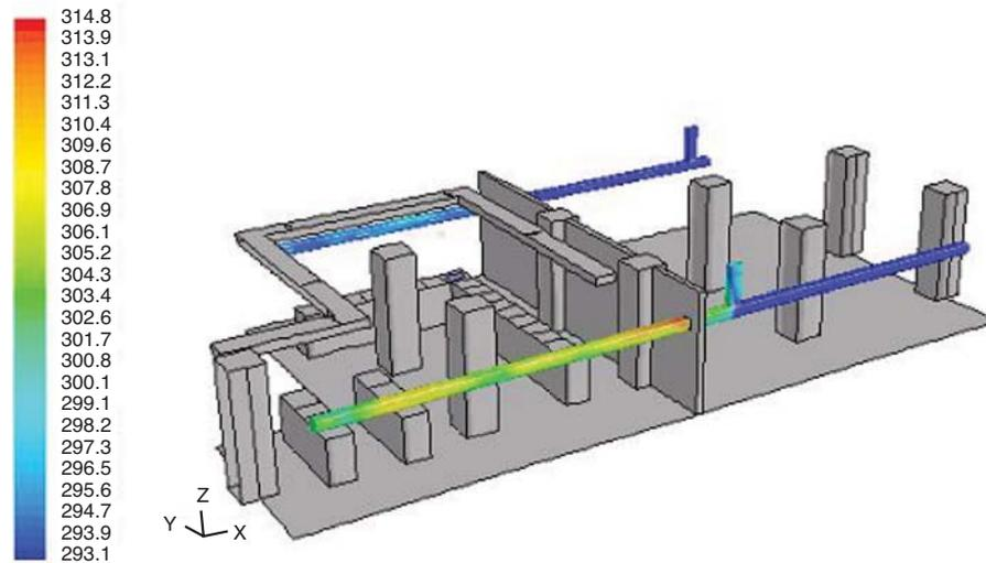
Fig. 3.31 - Maximum temperature in the ventilation ducts of ANS and SDS room and confining zone (long-term storage room)
