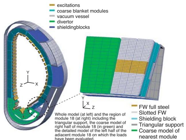
Fig. 3.6 - ITER model (EMAS code) after modifications made to accommodate the detailed model of module 18
