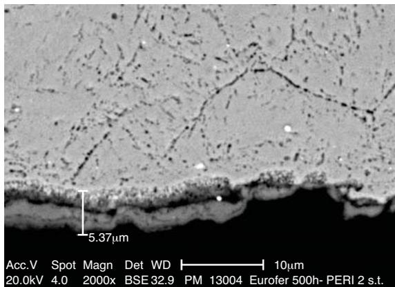
Fig. 3.7 - Surface micrograph of an oxidized specimen: the oxide layer produced by self-healing is evident
