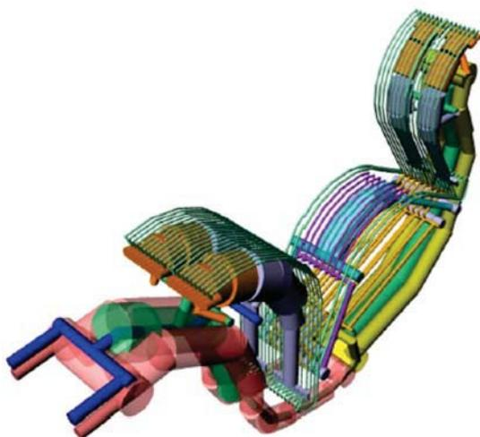
Fig. 3.2 - RELAP5: geometrical model of ITER divertor
