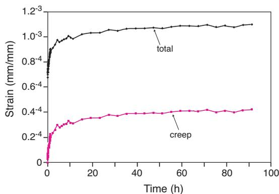
Fig. 3.24 - Total strain and creep strain vs. time
