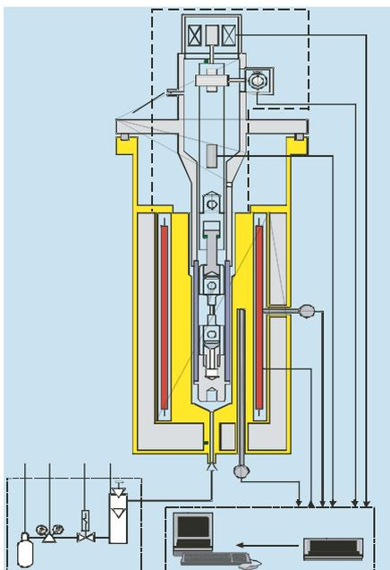
Fig. 3.8 - Tensile test machine for irradiated specimens
