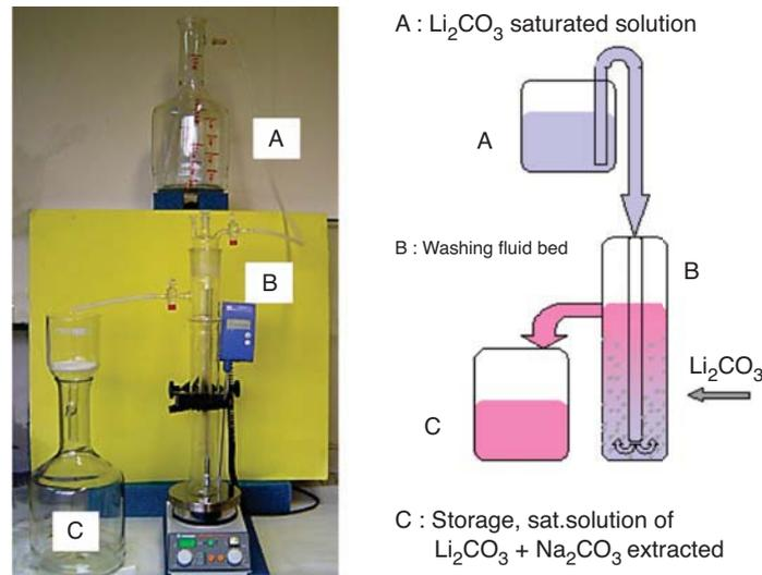
Fig. 3.10 - Schematic of the  $\text{Li}_2\text{CO}_3$  washing stage
