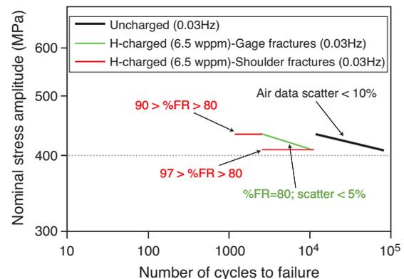
Fig. 3.25 - LCF curves of EUROFER 97 TGA weldment
