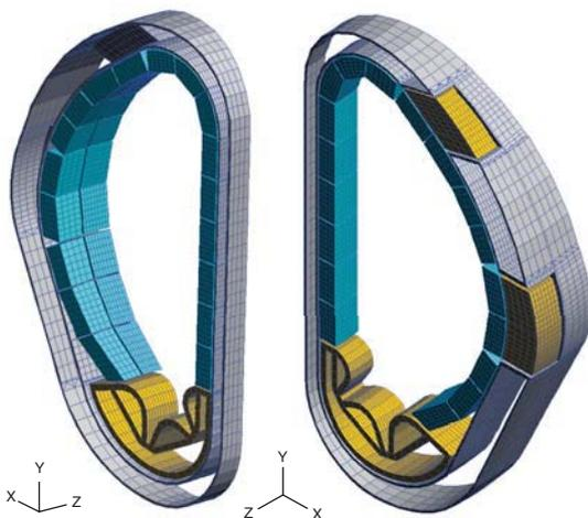
Fig. 3.5 - Coarse model (full 3D elements) of a  $10^\circ$  ITER sector including one half (two counter-faced halves) of the shielding blanket modules at the inboard (at the outboard), the double shell vessel and the main features of the upper and equatorial ports
