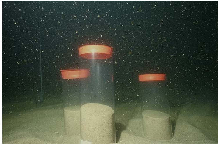
Photo 3. Collection of core samples.
