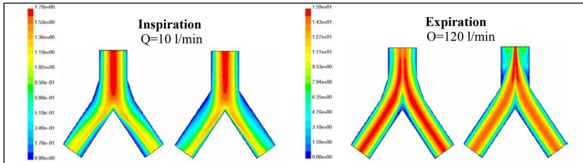
**Fig. 3** Flow fields for “narrow” and “wide” bifurcation models at 10 l/min flow rate, inspiration (left panel) and 120 l/min flow rate, expiration (right panel).
