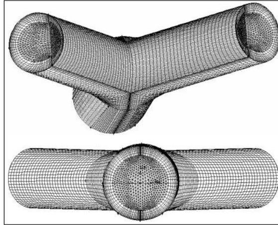
**Fig. 2** The numerical mesh used for airflow and trajectory calculations.
