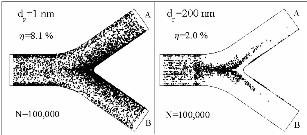
**Fig. 7** Deposition patterns of 1nm and 200 nm particles during inhalation at 60 l/min flow rate in an MRB bifurcation,  $d_p$ : particle size,  $\eta$ : deposition efficiency, N: number of particles.
