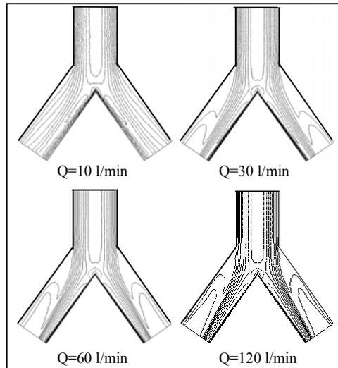
**Fig. 4** Flow fields at airway generations 3-4 at different tracheal flow rates. In each contour representation 10 velocity isolevels are displayed; a)  $Q=10$  l/min; b)  $Q=30$  l/min; c)  $Q=60$  l/min; d)  $Q=120$  l/min.
