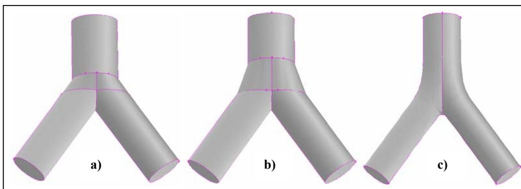
**Fig. 1** Bifurcation geometry models: a) “narrow”, b) “wide”, c) “MRB”
