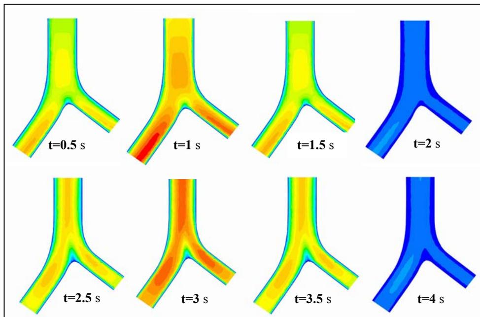
**Fig. 5** Some time dependent flow patterns in an asymmetrical bifurcation at 60 l/min flow rate during the second breathing cycle, inhalation (upper panel), exhalation (bottom panel), breathing cycle is 4 s.
