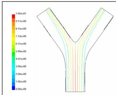
**Fig. 6** Trajectories of inhaled particles in a symmetrical MRB bifurcation model.
