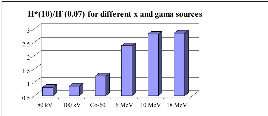
Figure 2: The dose ratio for TLD with two chips LiF exposed in Harshaw holders to  $^{90}\text{Sr}$
