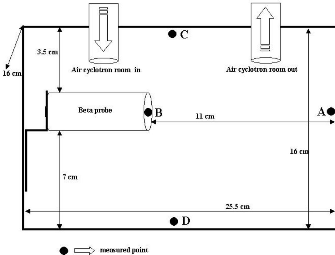
Fig.2 – detector set up for the cyclotron air contamination monitoring.
