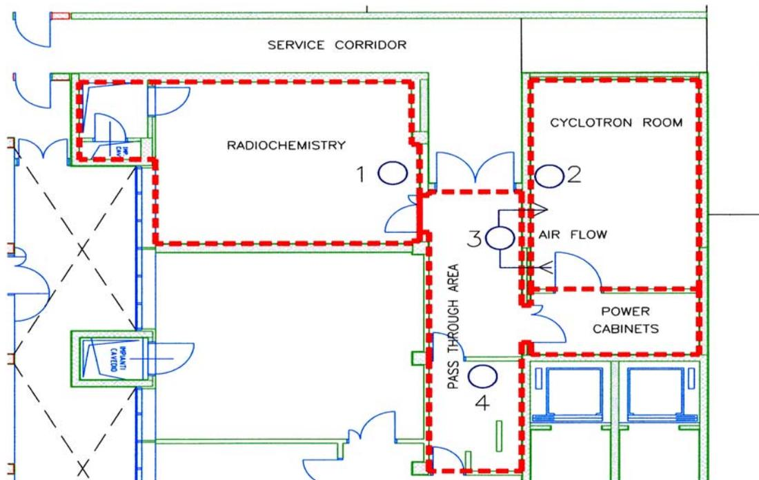
**Fig. 1** - location of the radioprotection monitors inside the installation
