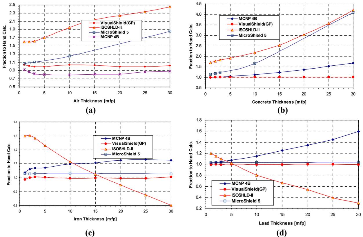
**Fig. 7. Comparison of dose rates resulting from a point source of 37GBq calculated with different tools. (a) and (b): air and concrete against 0.1 MeV photons, (c) and (d): iron and lead against 1 MeV photons.**
