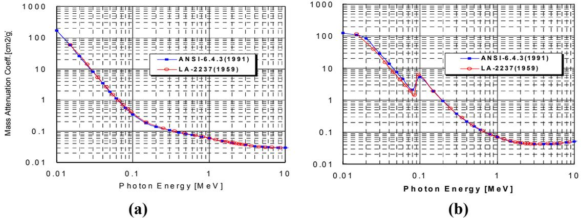
**Figure. 1. Mass attenuation coefficients for (a) iron and (b) lead.**
