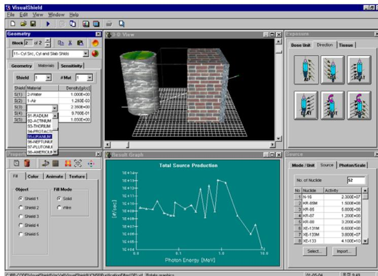
Figure 5. Main input window of VisualShield
