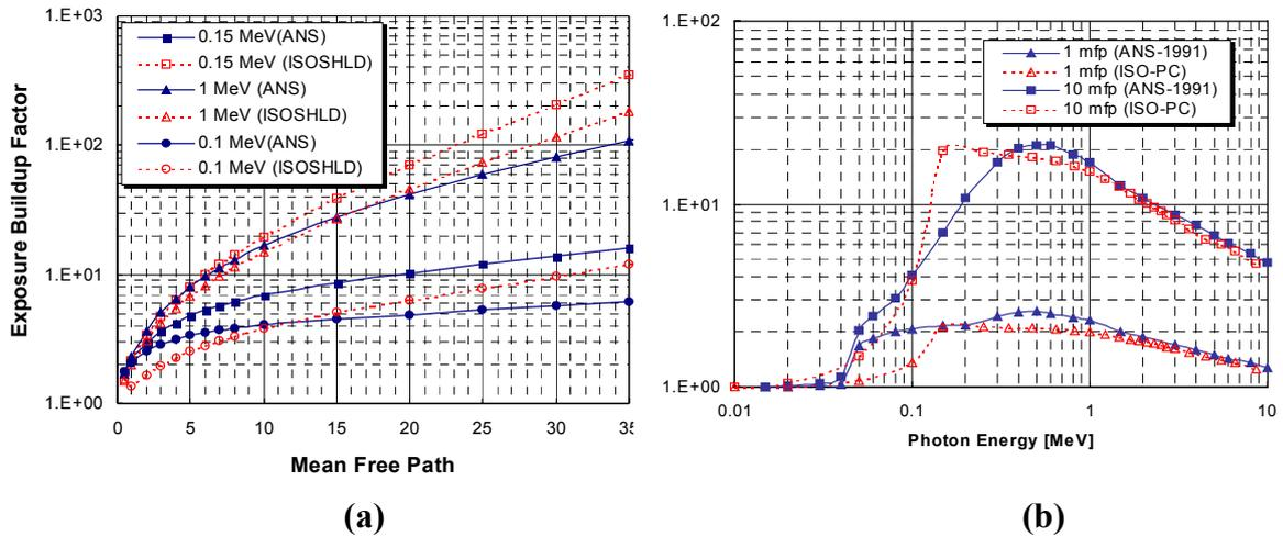
Figure. 2 Comparison of buildup factors for iron prescribed in ANSI/ANS with those used in ISOSHLD as a function of (a) shield thickness and (b) photon energy.
