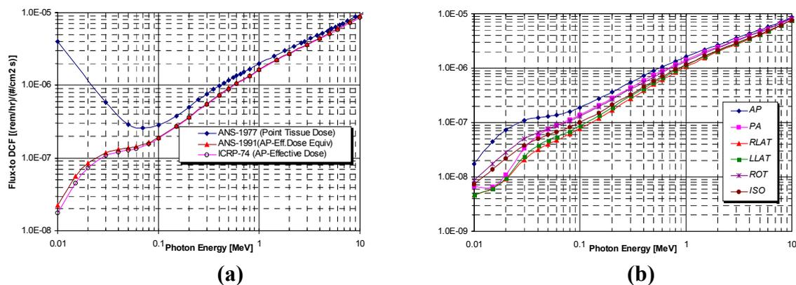
**Figure 4. Comparison of DCFs. (a) Point tissue dose DCF and effective doses, (b) Effect of irradiation direction on DCFs for effective dose, where AP denotes anteria-to-posteria, PA posteria-to-anteria, RLAT right lateral, LLAT left lateral, ROT rotational, and ISO isotropic irradiation conditions.**
