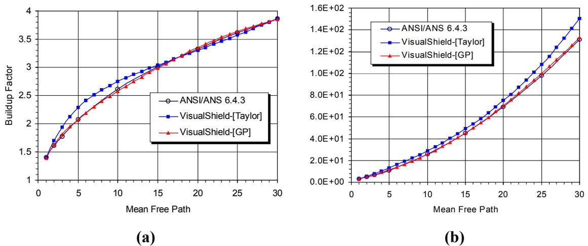
Figure. 3 Effect of the fitting functions on the buildup factors of 0.1 MeV photons (a) Iron (b) Concrete
