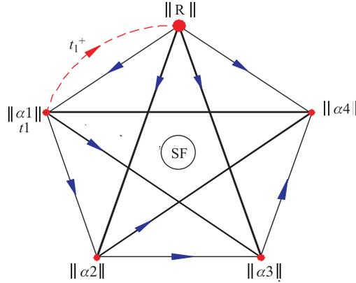
Fig. 6. Scheme of the more complete real-time algorithm to increase the efficiency of detection. Here  $R$  — recoil's matrix,  $\alpha_i$  — alpha particle matrix (Ref. [9, 10]). Loop  $t_1^+$  denotes writing, in the case of «unsuccess», of elapsed time for first alpha matrix to the recoil matrix cell
