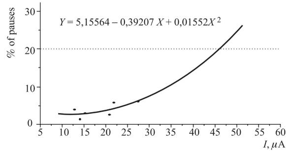
Fig. 2. The dependence of the typical total experimental efficiency loss value against incoming intensity of  $^{48}\text{Ca}$  ions. 20% loss level is shown by the dotted line. Second order (see Ref. [10]) polynomial fit is shown by the solid line. Polynomial second order fit is chosen as to be corresponding to «pessimistic» estimate of the upper level of the beam intensity
