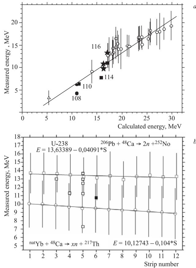
Fig. 3. *a*) Measured recoili energies are plotted against calculated ones. *b*) Measured recoil energies against strip number of the DGFRS PIPS detector for two reactions
