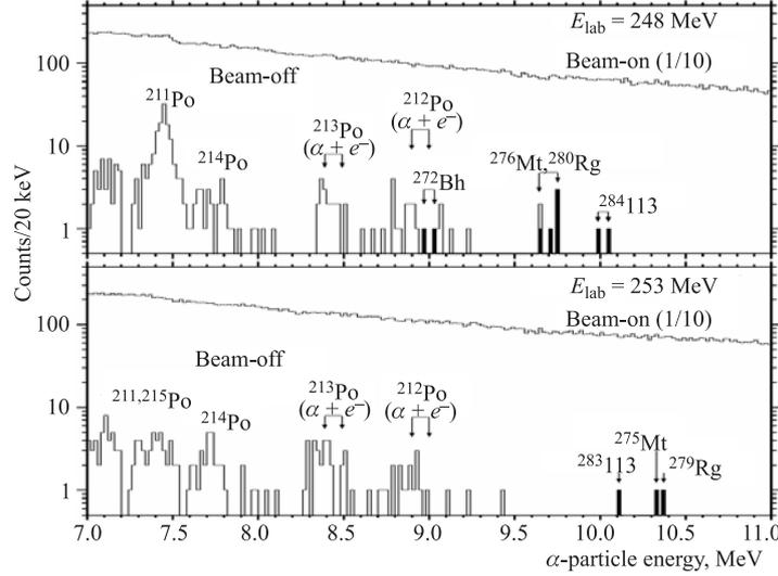
Fig. 4. Spectra of rare alpha decay events measured in  $^{243}\text{Am} + ^{48}\text{Ca} \rightarrow 115 + 3, 4 n$  experiment [2] at two beam energies (248, 253 MeV). The solid line shows background level — events which imitate alpha decays. Background suppression factor from 9 to 11 MeV region is estimated as  $\sim 10^5$
