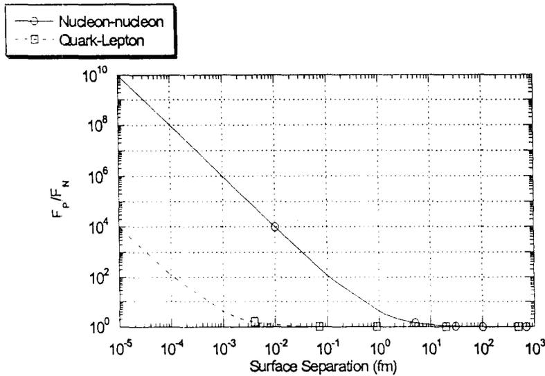
FIGURE 2. Ratio of modified force to Newtonian gravitation as a function of surface separation for nucleon-nucleon and quark-lepton interactions. The ratio approaches unity at large surface separations in both cases. Also, for both interactions the ratio becomes quite large for short separations, reaching  $10^{40}$  for the nucleon-nucleon interaction and  $10^{34}$  for the quark-lepton interaction in the Planck length separation limit of  $10^{-20}$  fm.
