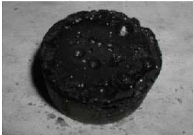
Fig. 11. After electrolysis of LiI in LiCl salt with 200 and 250mA reduction current.
