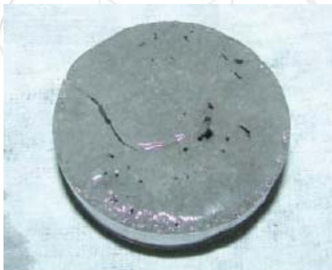
Fig. 7. Electrolysed LiCl salt of LiBr after washing with water.
