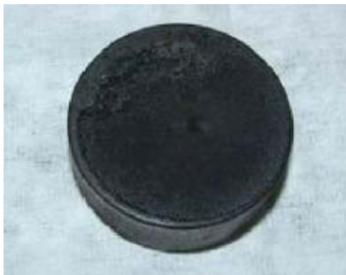
Fig. 6. Electrolysed LiCl salt of 3wt% LiBr with 100mA reduction current.
