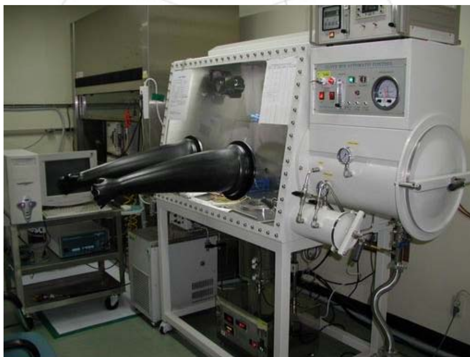
Fig. 1. Glove box for the Electrochemical Measurement.
