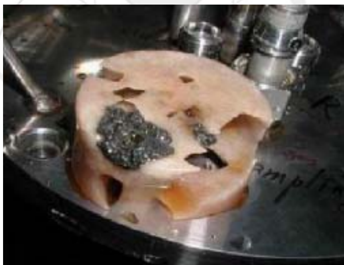
Fig. 16. Precipitates after the electrolysis of Li 2 Se in LiCl with 400mA current for 1 hour.
