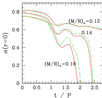
Figure 4: The lapse function  $\alpha$  at  $r = 0$  as a function of coordinate time for models (A)–(C). The solid and dashed lines denote the results for simulations with  $293 \times 293 \times 147$  grid resolution and with  $193 \times 193 \times 97$  grid resolution. For smaller scale simulations, the grid size is  $116/96$  times larger than that for larger scale simulations. (Namely, the outer boundaries along each axis are located  $116L/146$  in these cases.)
