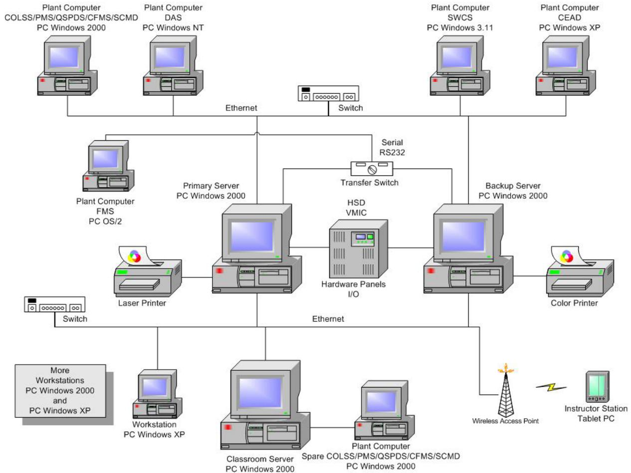
**Figure 2: SONGS Simulator Architecture following Re-host**
