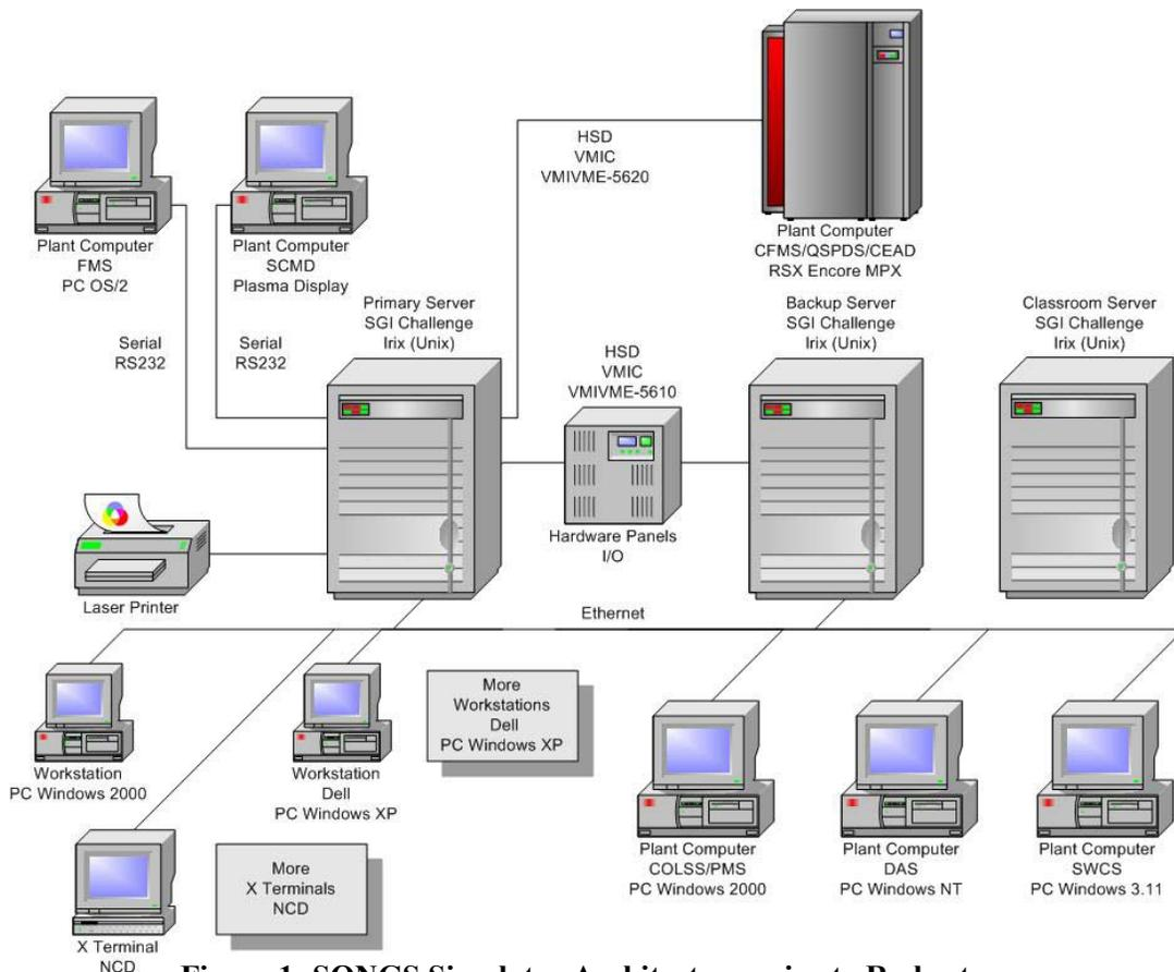
Figure 1: SONGS Simulator Architecture prior to Re-host
