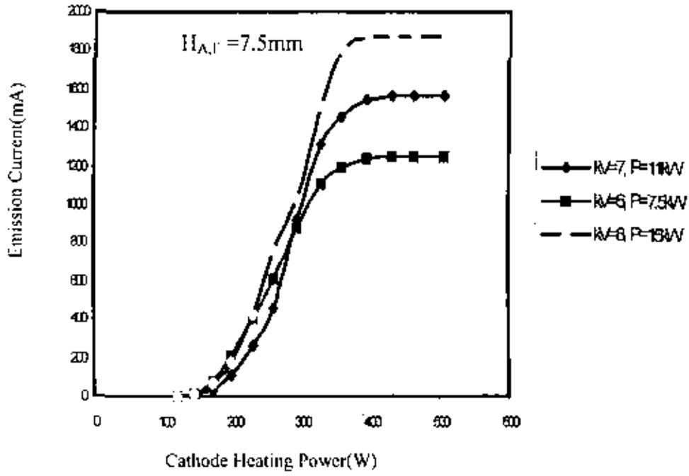
Fig.13: Emission Characteristics of LS Emitter Assembly
