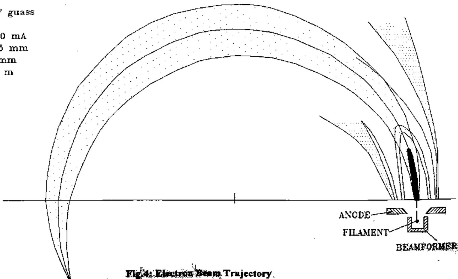
**Fig. 4: Electron Beam Trajectory.**
