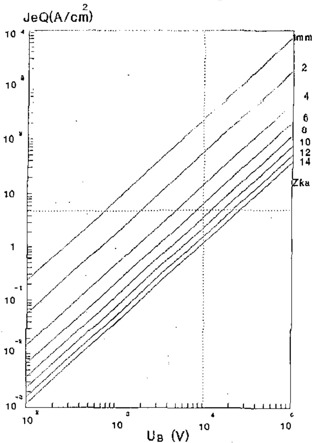
Fig. 7: Emission Current (Space Charge Limited) Vs Acceleration Voltage
