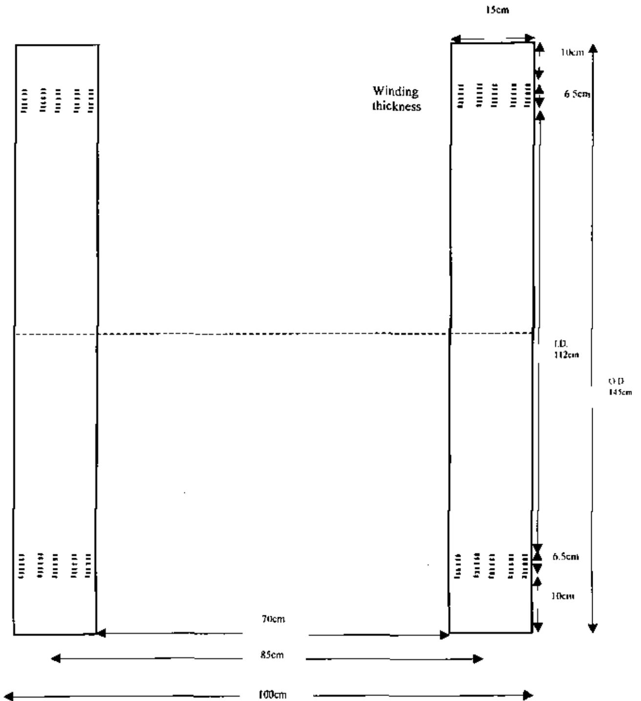
**Fig.3: Large Diameter Helmholtz Coil**
