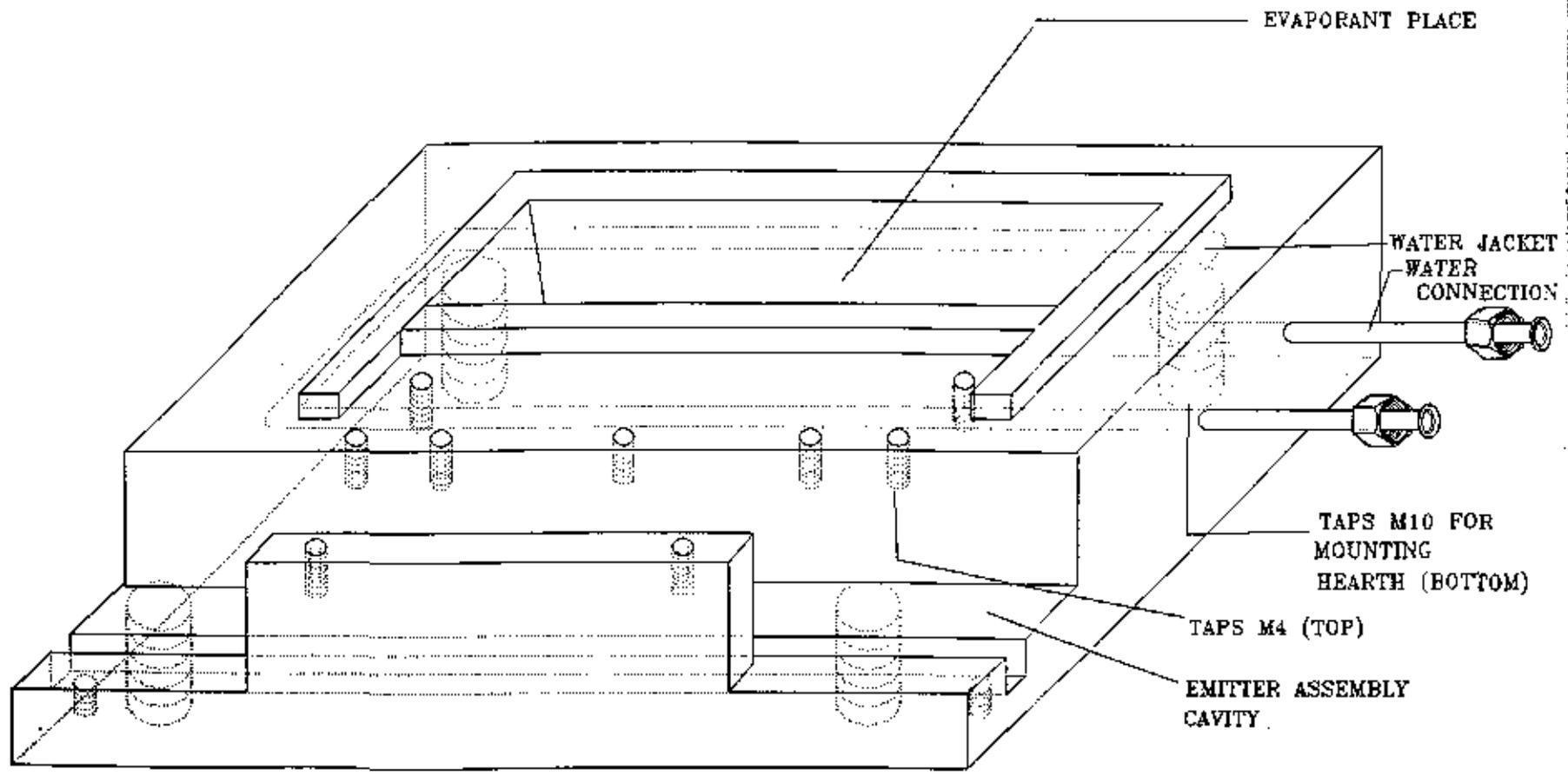
**Fig.8: Water Cooled Copper Hearth**
