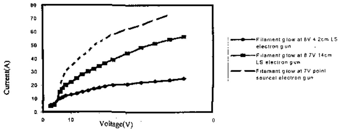
**Fig.11: Voltage Current Characteristics**
