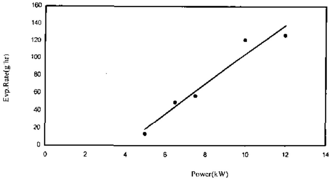
**Fig. 9(a): Evaporation Rate Vs Power at  $H_{a,z} = 7.5\text{mm}$**
