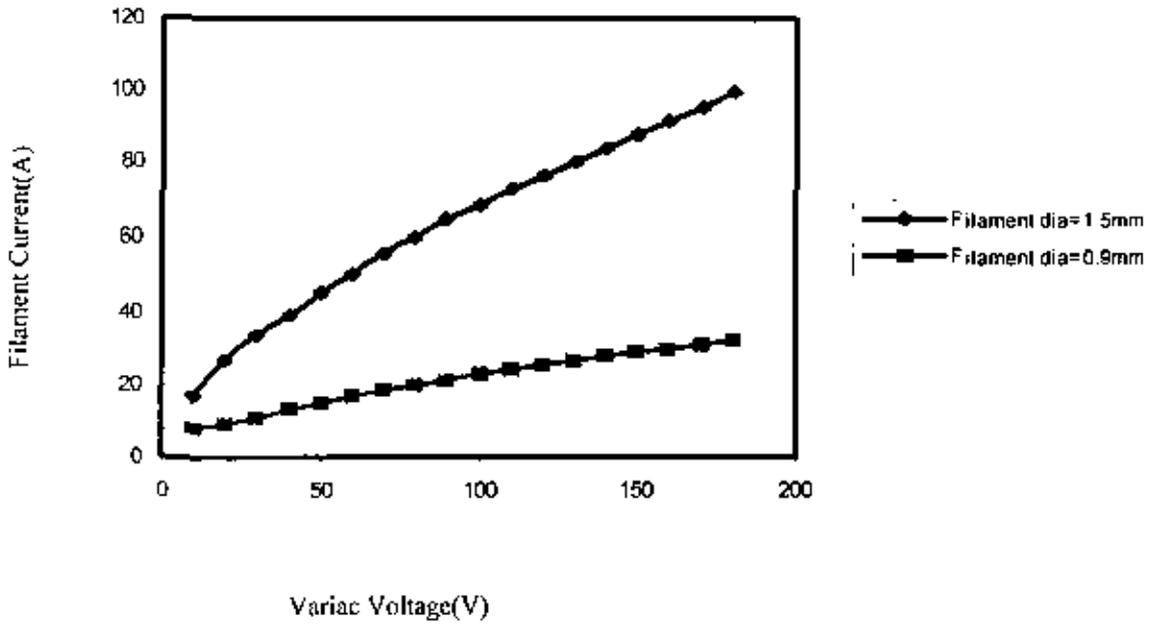
Fig. 12: Filament Current Vs Variac Voltage
