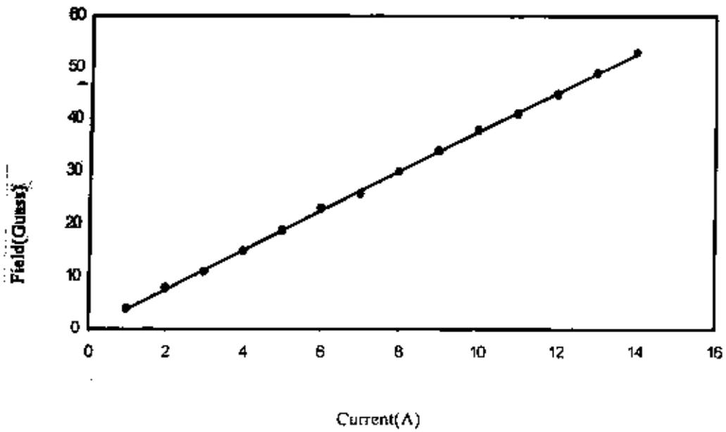
**Fig.1: Magnetic Field at the Centre of the Coil**
