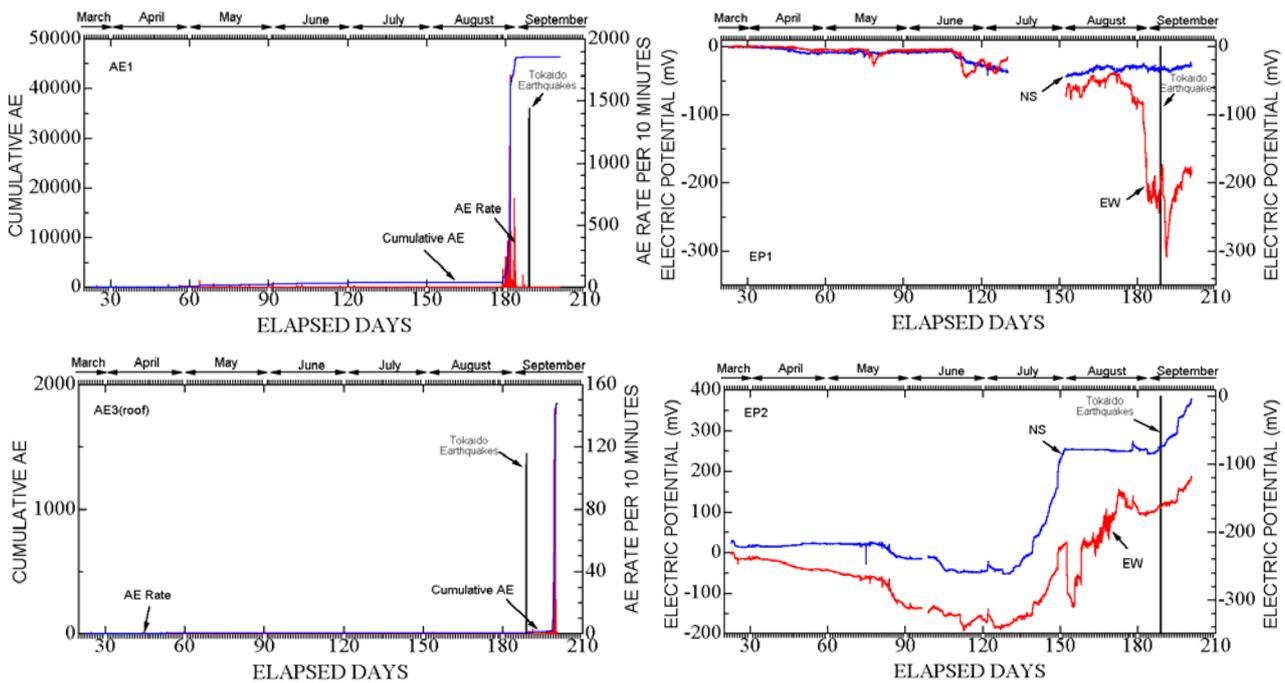
Figure 8: Variations of geo-electric potential and acoustic emission (AE) counts
