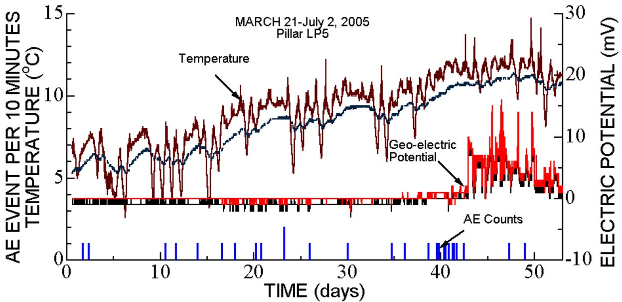
Figure 11: Multi-parameter response of Pillar LP5 during March 21 and July 02, 2005
