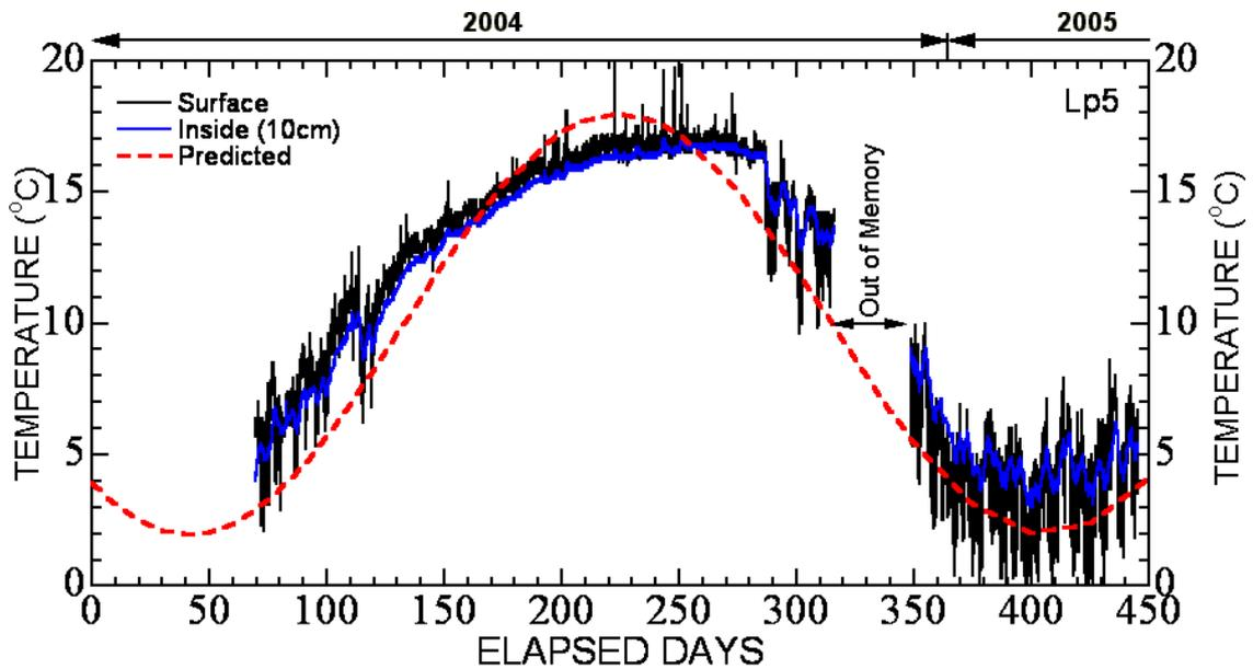
Figure 6: Variations of temperature on the surface and inside pillar denoted LP5
