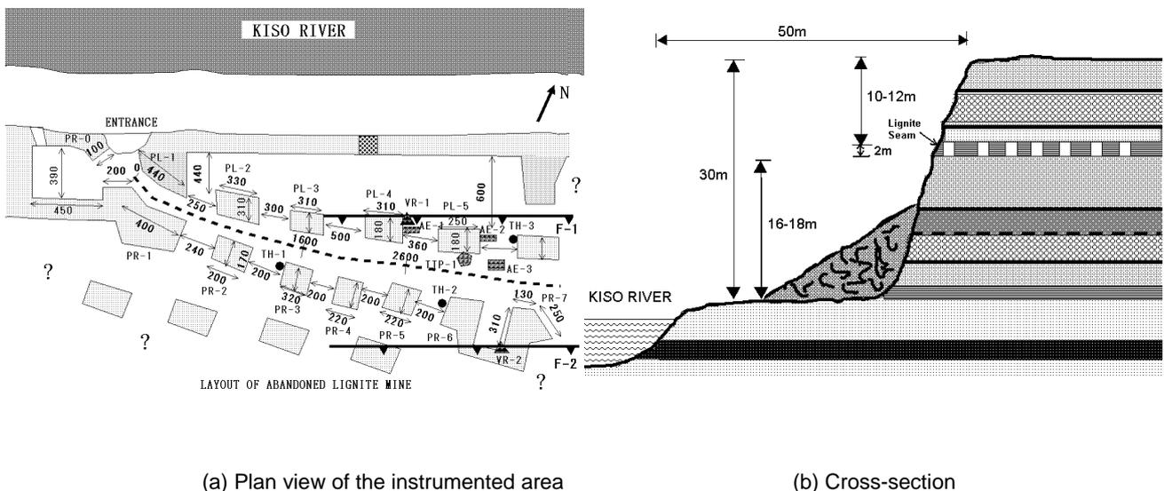
Figure 1: Plane view of the instrumented area of the abandoned mine and a typical cross-section
