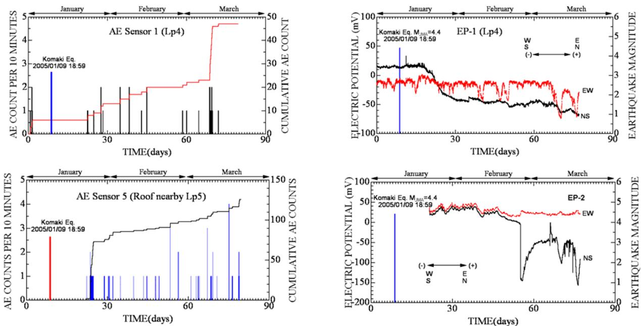
Figure 9: Variations of geo-electric potential and acoustic emission (AE) counts
