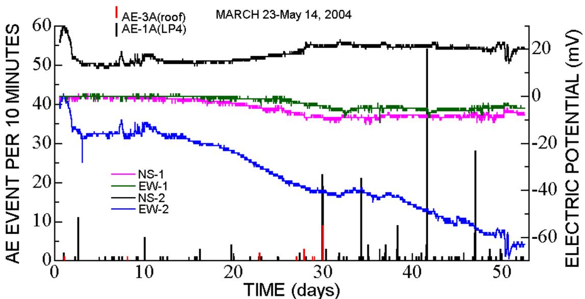
Figure 7: Variations of geo-electric potential and acoustic emission (AE) counts
