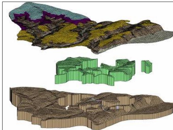
Figure 8. Liège coal basin pilot site. Mixed approach. In brown parts modelled with FE elements, in green the five parts considered as box
