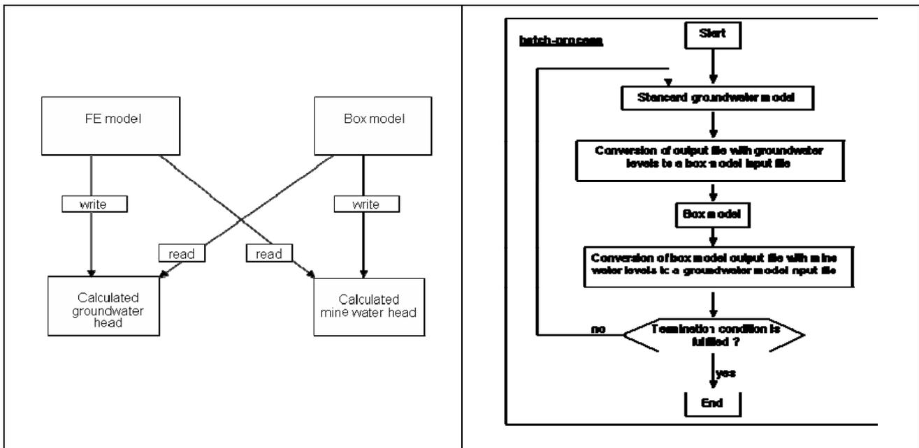
Figure 4. Schematic flow diagram of the FE-Box model coupling by batch process
