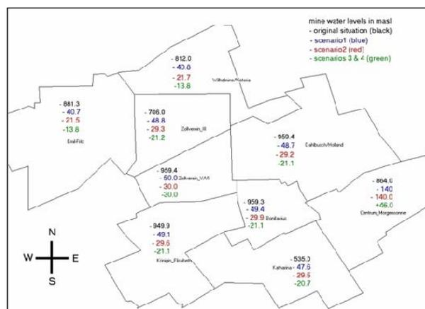
Figure 6. Schwartzbach pilot site. Mine water levels in the different boxes of the Emschermulde model according to the final pumping level
