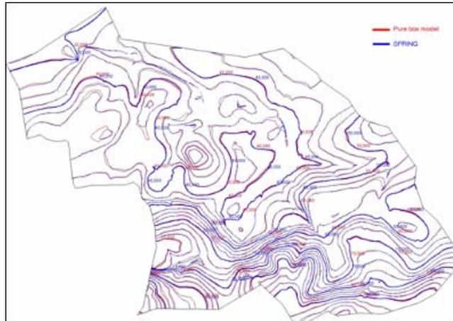
Figure 5. Schwartzbach pilot site. Comparison of groundwater contour lines of the pure box model simulating the present situation with those of the SPRING model
