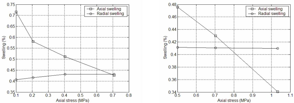
Figure 5. Axial swelling and radial swelling versus axial stress
