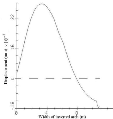
Figure 15. Normal displacement to invert (mm)
