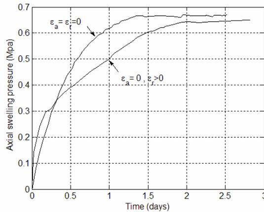
Figure 4. Swelling pressure versus time for two different lateral confinement
