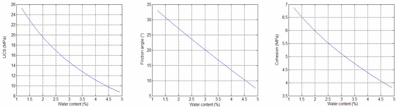
Figure 3. UCS, friction angle and cohesion versus water content
