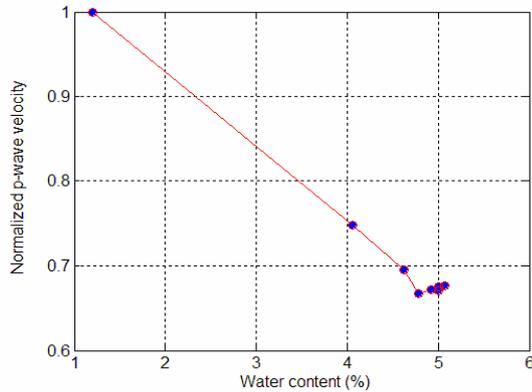
Figure 1. Normalized p-wave versus water content
