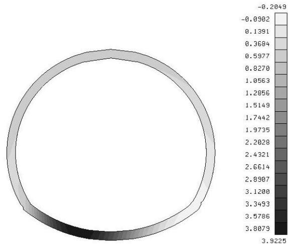
Figure 14. Vertical displacement of lining (mm)
