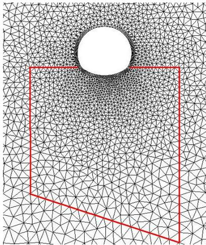
Figure 13. Detailed of the mesh used in modelling
