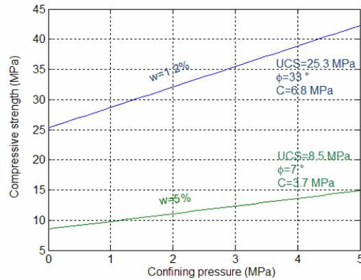
Figure 2. Mohr-Coulomb failure criteria for two water contents
