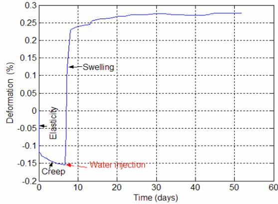
Figure 7. Three phases of deformation
