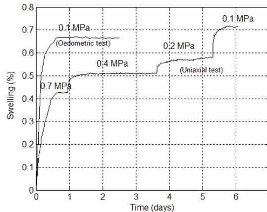
Figure 6. Comparison between uniaxial test and oedometric test for 0.1 MPa of axial stress
