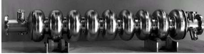
Figure 1: Superconducting 1.3 GHz 9-cell cavity for the TESLA Test Facility [2].
