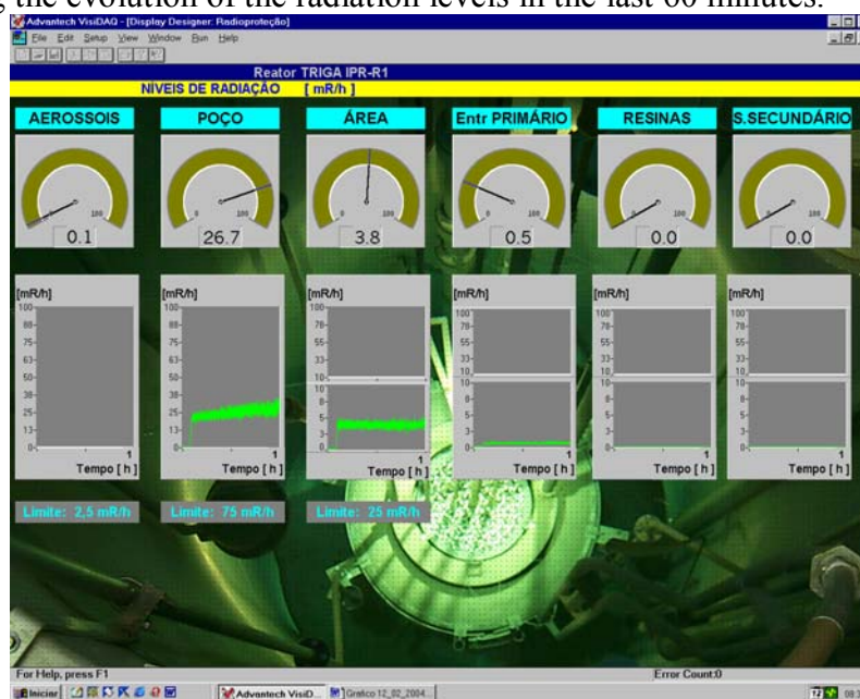
Figure 5 – Radiation Monitoring System
