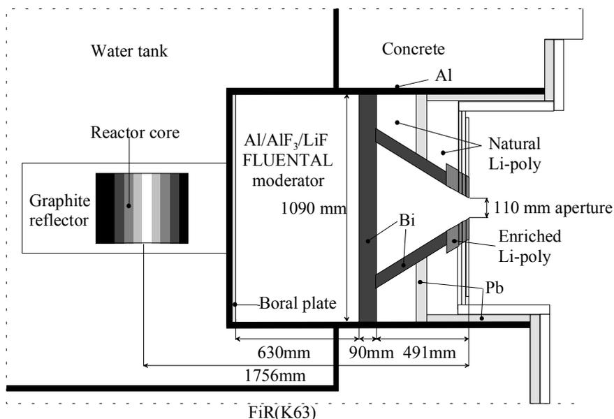
FIG. 2. The epithermal neutron irradiation facility in its current configuration with a 63 cm thick FLUENTAL™ moderator. In patient treatments normally 14 and 11 cm diameter beams are used.
