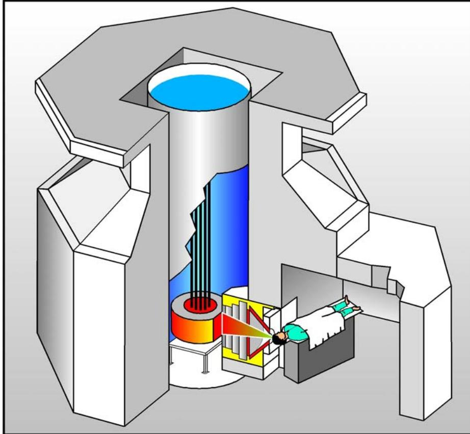
FIG. 1. BNCT Facility at the FiR 1 –reactor.
