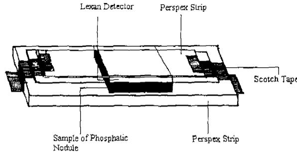
Fig. 2. Diagrammatic sketch showing packing assembly for irradiation of phosphatic nodules at Pakistan Research Reactor – I through a rabbit station at 10 MW power.
