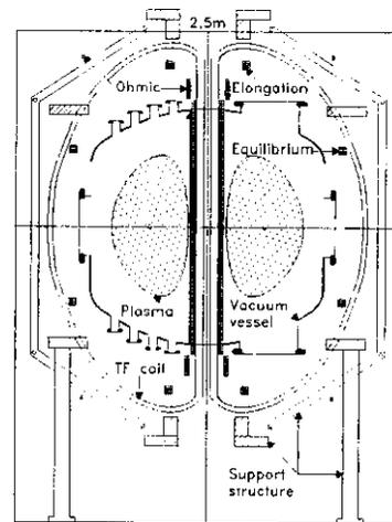
Figure 11. Cross-section of the ETE tokamak.
