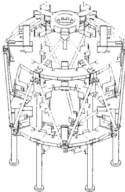
Figure 13. Structure for supporting the vacuum vessel] and coils of ETE.
