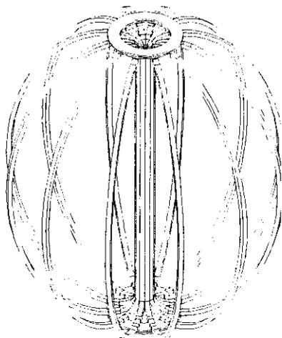
Figure 6. Toroidal field coil of the ETE tokamak.
