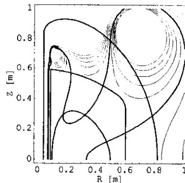
Figure 12. Magnetizing flux contours on the poloidal plane. The heavy contour indicates a poloidal flux of 0.25Wb (2x7.8MA-turns in the OH solenoid for double-swing operation) with a 2% increment between contours. The plasma outline, and the vacuum vessel and toroidal field coil centerlines are also displayed.
