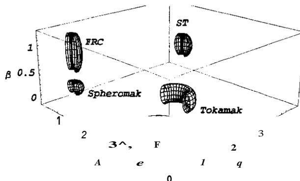
Figure 2. Axisymmetric configurations. Spherical tokamaks present both the strong toroidicity effects of compact tori (notably magnetic shear) and the good stability properties provided by the external toroidal field of conventional tokamaks.
