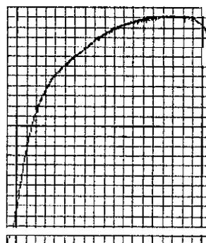
Figure 9. Stress-strain diagram for the external (superposition) demountable joint of the TF coil. Each horizontal division corresponds to a displacement of  $1\text{ mm}$  and each vertical division to a force increment of  $3.07\text{ kN}$ .
