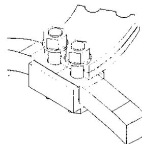
Figure 8. Single bolt demountable joints of the TF coil.
