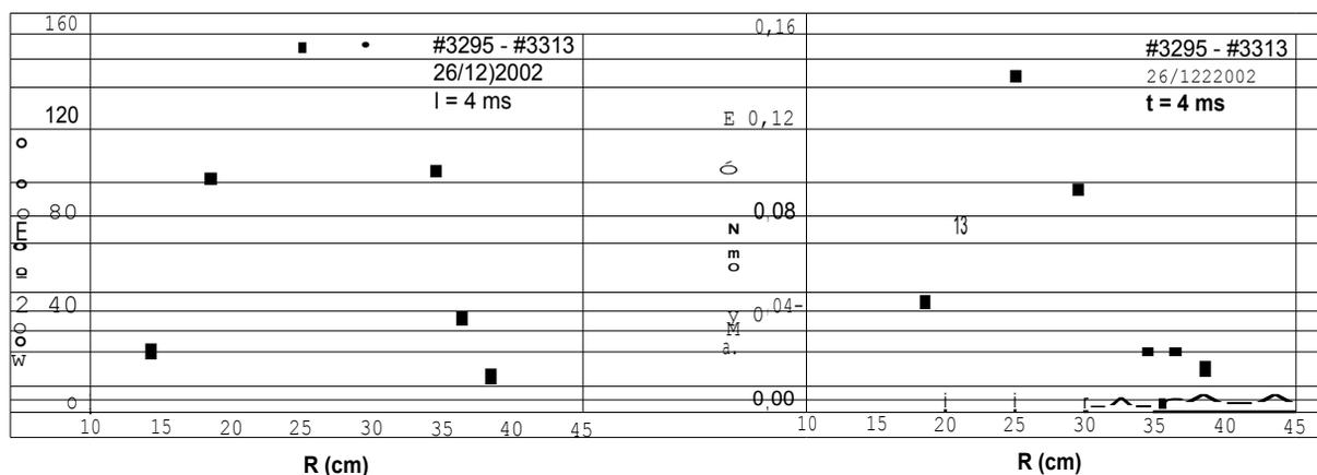
Figure 19. Radial distribution of the electron temperature 4ms after the start of the discharge in ETE.
