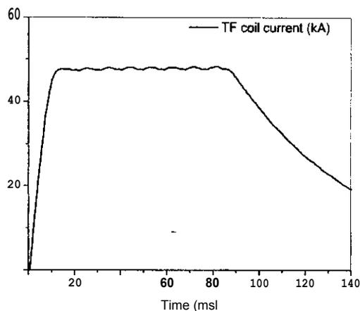
Figure 14. Current waveform in the TF coil, obtained by numerical simulation.
