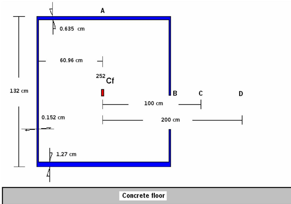
Figure 2. Monte Carlo model of WEP shield structure.
