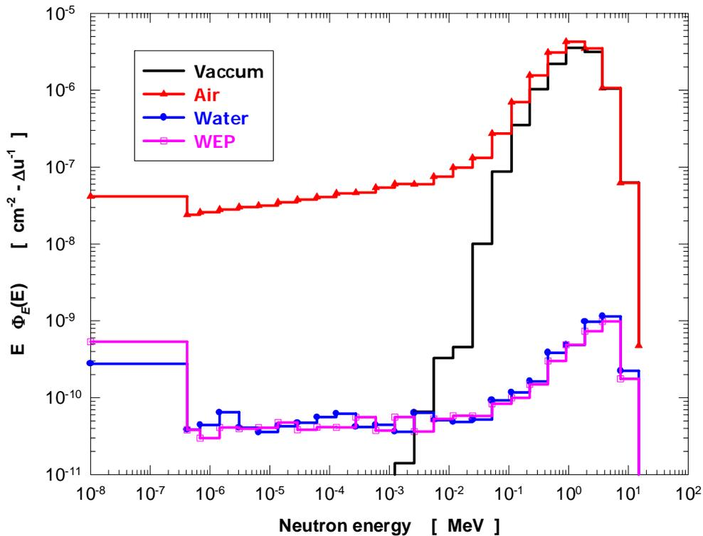
Figure 5. <sup>252</sup>Cf neutron spectra at site C.
