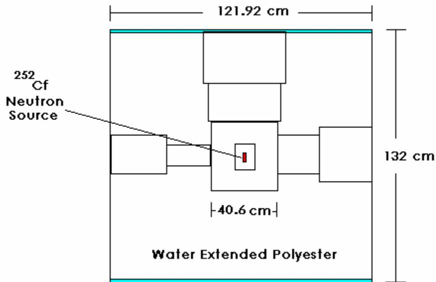
**Figure 1. NETL WEP neutron shielding**
