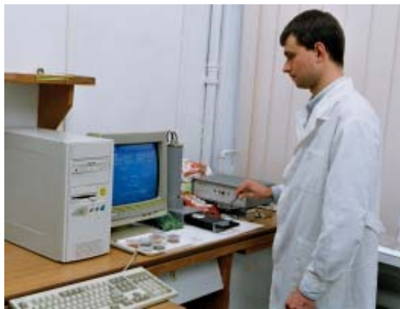
Fig.1. Irradiated Food Screening System SURRC PPSL installed in this Laboratory. Placing of a Petri dish with a sample inside into a sample chamber by means of tweezers.
