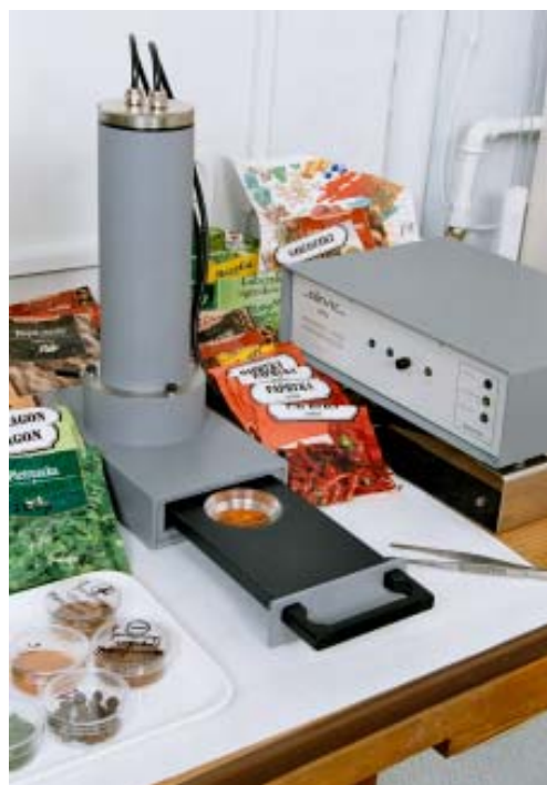
Fig.3. Irradiated Food Screening System SURRC PPSL installed in this Laboratory. From the right to the left: control unit and detector head assembly with sample chamber. Note three colour diodes (red, amber, green) on front panel of control unit.
