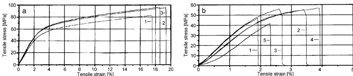
Fig.2. Samples of tensile measurements results of PET membrane: a) initial and b) after 52 h UV irradiation.
