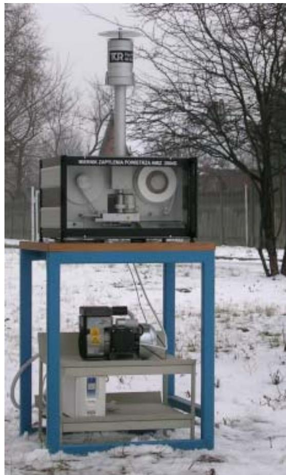
Fig.1. Airborne dust concentration gauge AMIZ-2004G.
