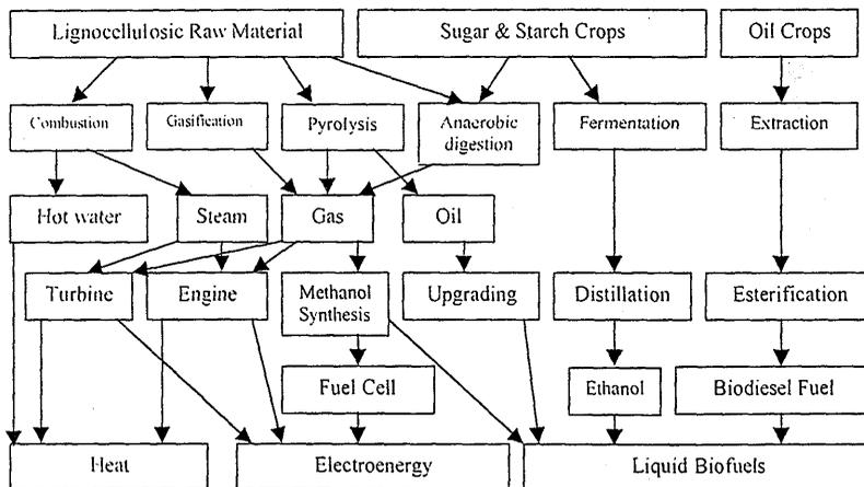
Figure 1. Possible converting of biomass to end-products
