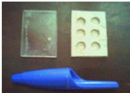
*Figure 1: Acrylic plate and perforated cardboard*
