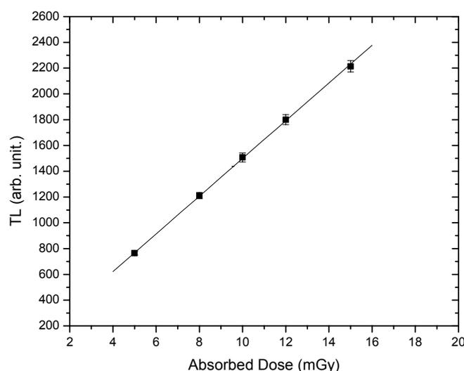
**Figure 3: Calibration curve of monitors when irradiated with gamma rays ( $^{60}\text{Co}$ ).**
