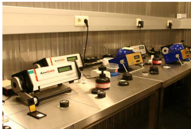
Fig. 1: Radon measuring instruments and detectors placed in the radon calibration laboratory, BEV Arsenal, Vienna
