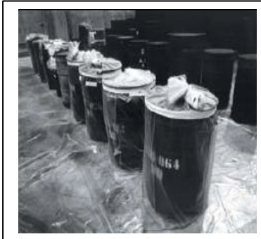
figure 5: a limited number of bitumized waste drums, with outflow of the non-active bitumen matrix, are put a side to perform a continous follow-up of the state of the drums
