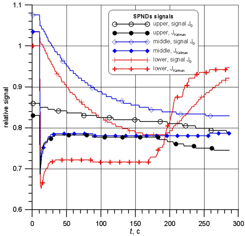
**Figure 3. SPNDs signals in the cell 29 in course of the process with rod drop, ‘as it is’ and with Kalman filter processing.**
