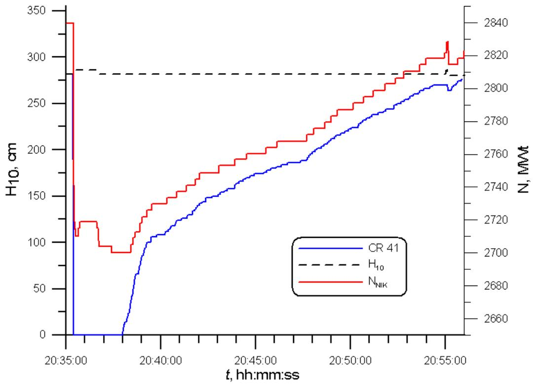
**Figure 2. Control rods position and the core neutron power (by ex-core detectors) in course of the process with rod drop.**
