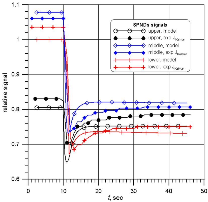
**Figure 5. Neutron flux in the SPND location in the cell 40 in course of the process with rod drop, SPND signals with Kalman filtering and results of modelling.**
