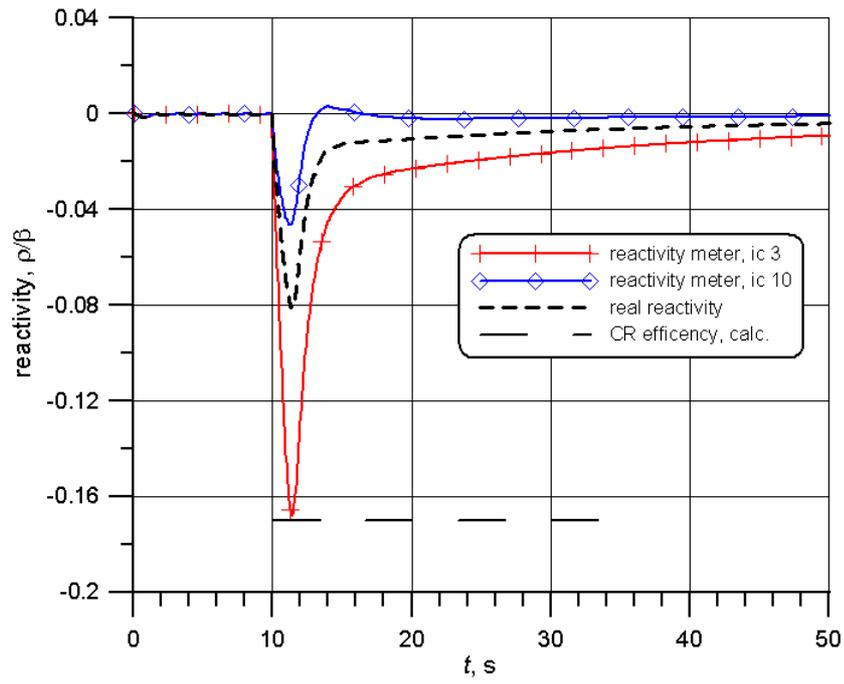
**Figure 6. Rod drop process imitation. Reactivity history by the readings of ex-core ion chambers, by the 3D dynamic calculation; CR calculated efficiency.**
