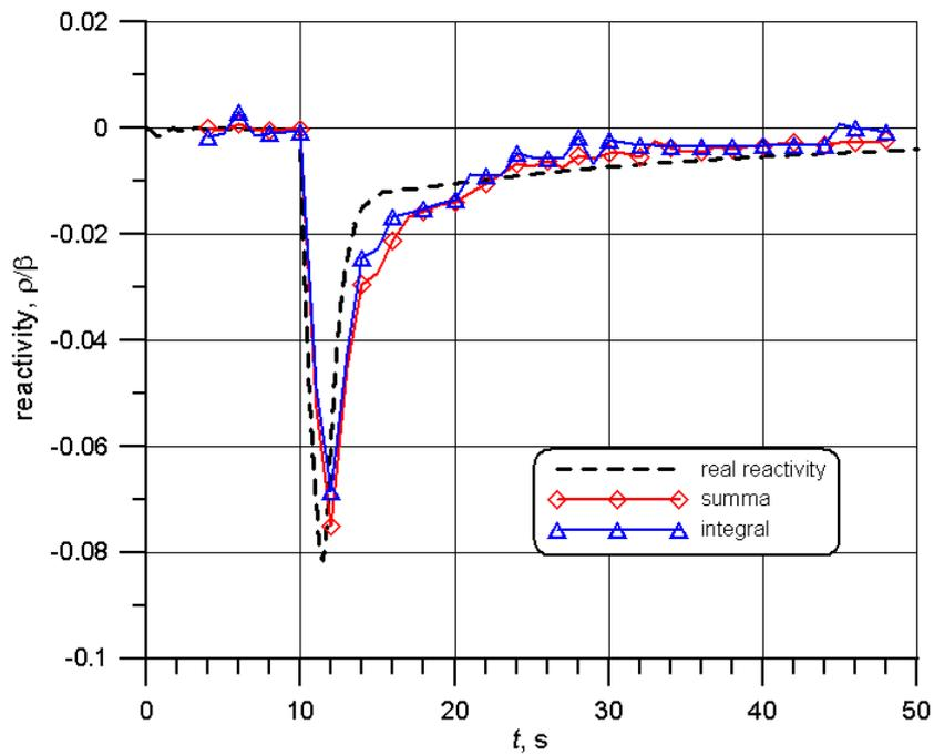
**Figure 7. Reactivity history in course of the process with rod drop, obtained by dynamic calculation, and by processing of the integral signal of all SPNDs with Kalman filter.**
