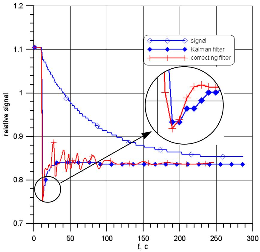
**Figure 4. SPND signals in the cell 30 in course of the process with rod drop , ‘as it is’, with Kalman filter processing, with corrective filter processing.**
