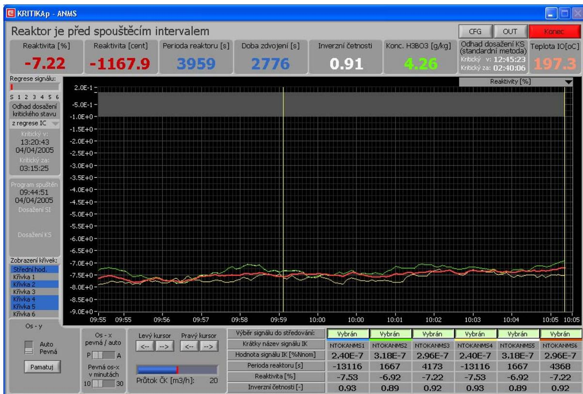
Figure 3: Module for monitoring of approaching to reactor critical state (Dukovany NPP).
