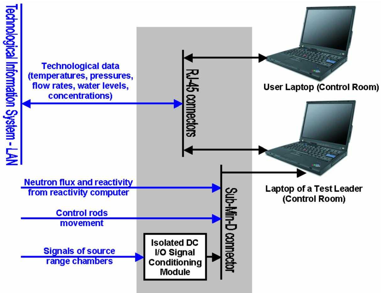
Figure 1: Basic wiring diagram of mobile Innovated Non-Standard Measurement System iNMS for Bohunice NPP (Slovak Republic).
