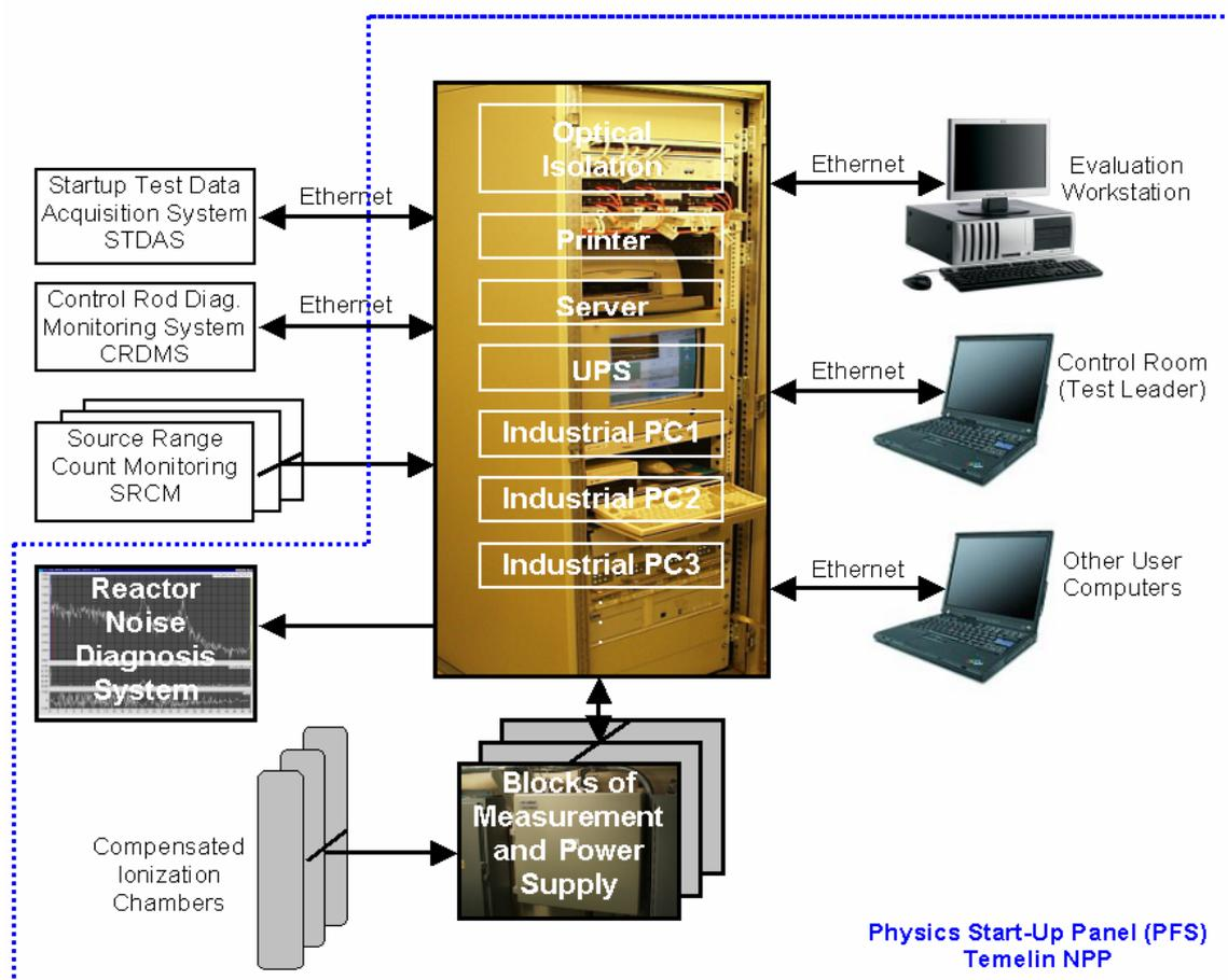
Figure 2: Basic wiring diagram of stationary measurement and evaluation system Physics Start-Up Panel at Temelin NPP (Czech Republic).
