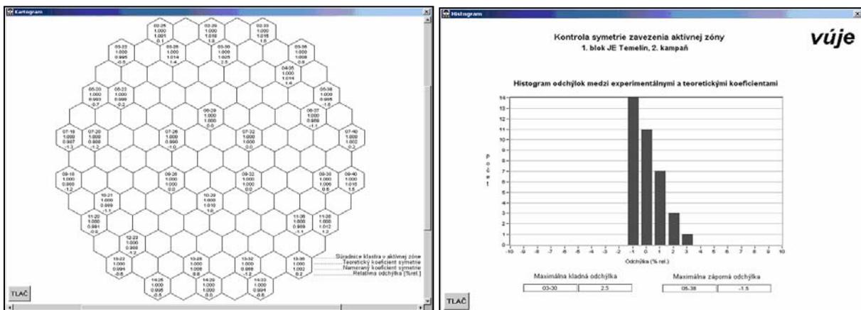
Figure 5: Screenshots of the module for measurement of reactor core symmetry.
