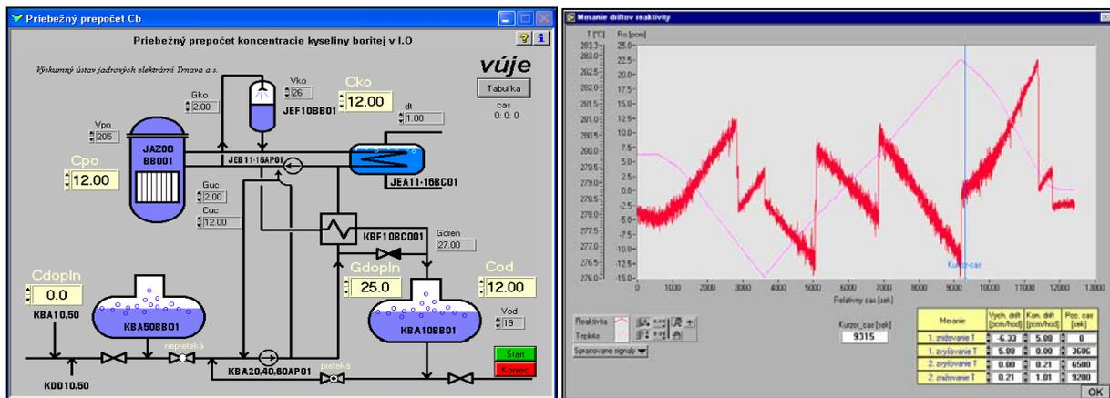
Figure 4: Module for simulation of boric acid concentration changes in primary circuit (left) and module for evaluation of temperature coefficient (right).
