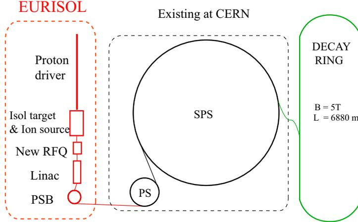
Figure 12: A schematic layout of the BetaBeam complex. On the left, the low energy part is largely similar to the EURISOL project [33]. The central part (PS and SPS) uses existing facilities. On the right, the decay ring has to be built.
