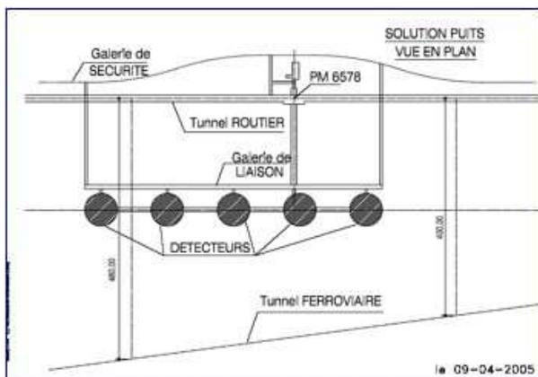
Figure 2: Possible layout of the Fréjus underground laboratory.
