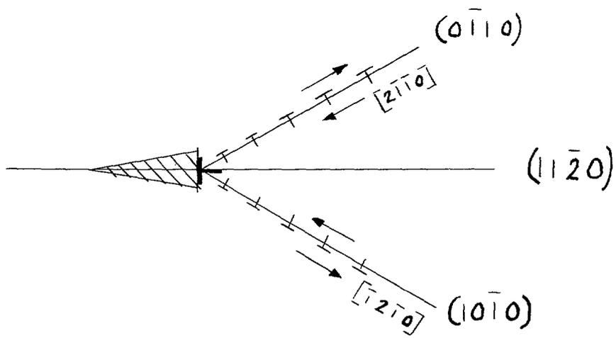
Fig. 3. Model for crack nucleation along  $\{11\bar{2}0\}$ .
