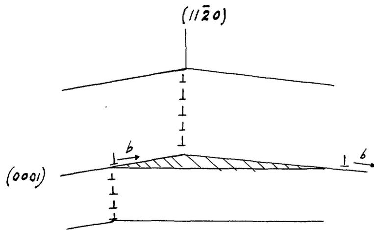
Fig. 2. Model for crack nucleation along  $(0001)$ .
