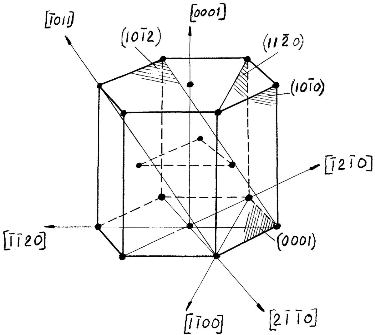
**Fig 1.** Crystallographic planes and directions in hexagonal close-packed metals.
