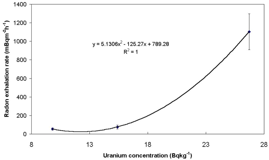
Fig. 2 Dependence of radon exhalation rate on the uranium concentration for marble
