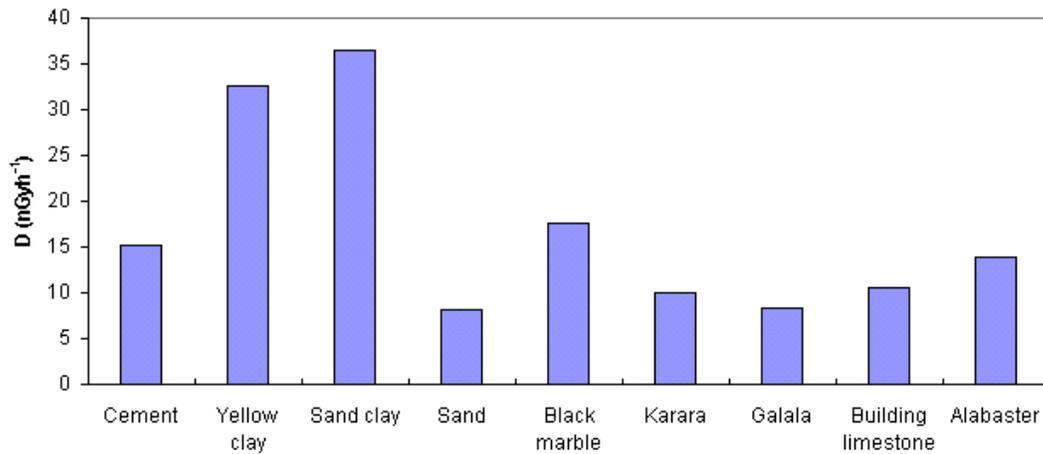
**Fig. 4 The variations of absorbed dose rate in air ( $D$ ) in  $\text{nGy h}^{-1}$  for alabaster, marble, raw building bricks and building limestone**
