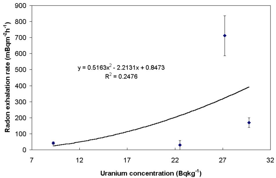
Fig. 3 Dependence of radon exhalation rate on the uranium concentration for raw of building bricks.
