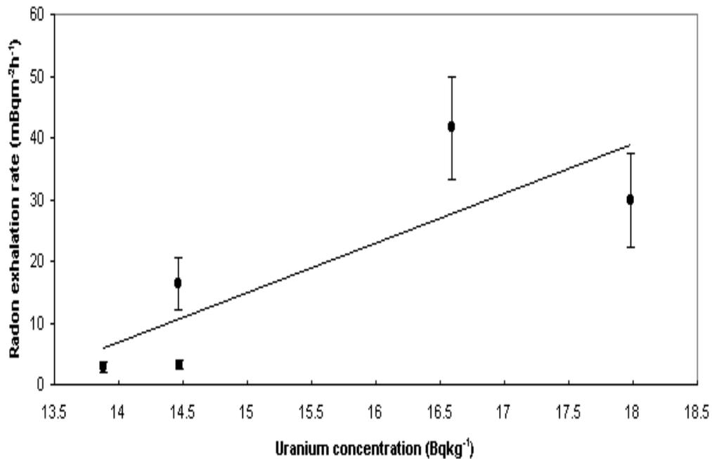
**Fig. 1 Dependence of radon exhalation rate on the uranium concentration for alabaster samples.**
