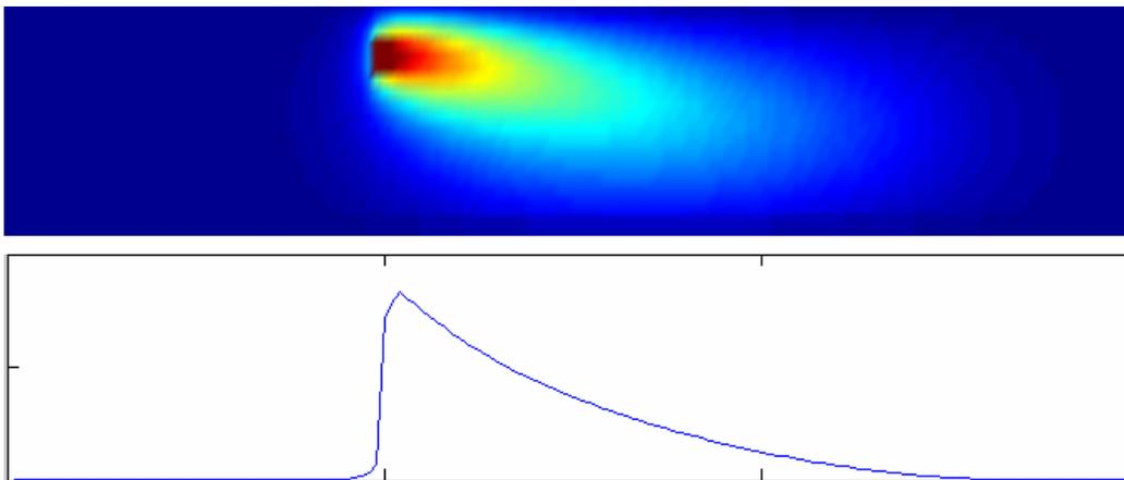
Figure 1.- Tracer distribution and standard deviation (without obstacles).
