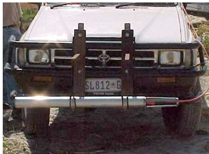
Figure 3. The MEDUSA detector fitted on a 4×4 vehicle for gamma-ray measurements on the gold-mine tailings dam.
