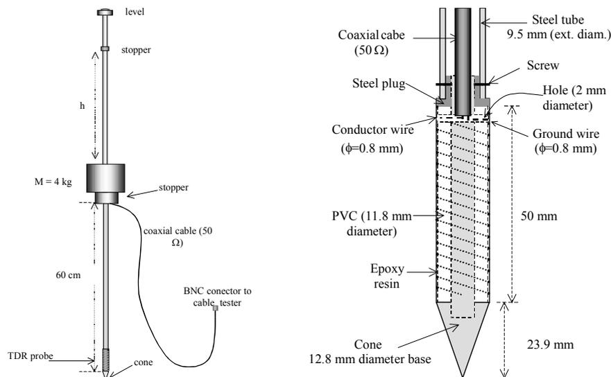
Figure 1. Combined penetrometer – coiled TDR moisture probe.
