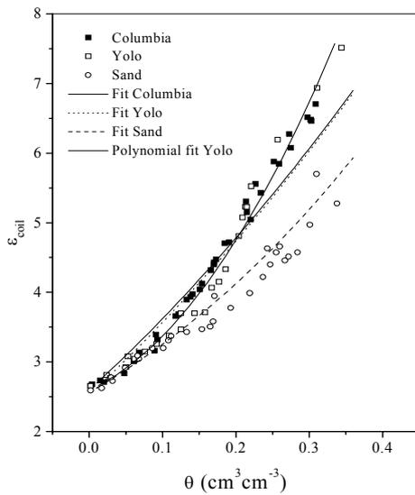
Figure 3. Calibration data for the coiled TDR probe using Eq. [3] for 3 soils, using parameters  $n$ ,  $w$ ,  $\epsilon_{probe}$  fitted to Eq. [1] and soil specific  $\alpha$ -values fitted to Eq. [2].
