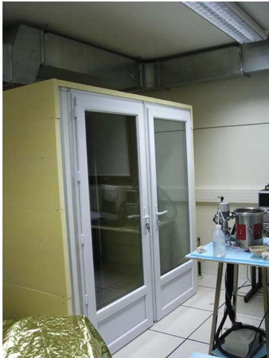
Figure 13. A temperature stabilized cabin was built in the laboratory to solve the problems of temperature stability of the environment, and to allow for measurements at different temperatures. The vacuum chamber, not yet installed into the cabin, is seen to the right.
