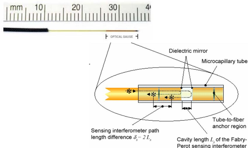
Figure 1: Schematic view of an Extrinsic Fabry-Pérot Interferometer and its working principle. [G. Daplain, technologie interférométrie en lumière blanche, [www.opsens.com](http://www.opsens.com)]
