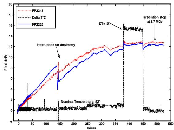
Figure 3: Evolution of the central wavelength drift (expressed in pixels) as a function of the irradiation time (up to 8.7 MGy). 1 pixel corresponds to a 9 nm change in the Fabry-Pérot cavity length.
