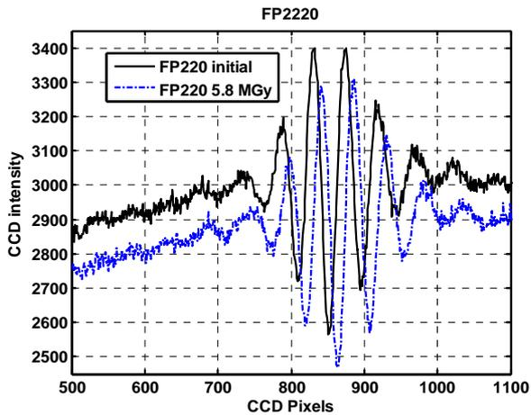
Figure 2: Comparison of the interferogram of a EFPI before (solid line) and after (dashed line) gamma irradiation.
