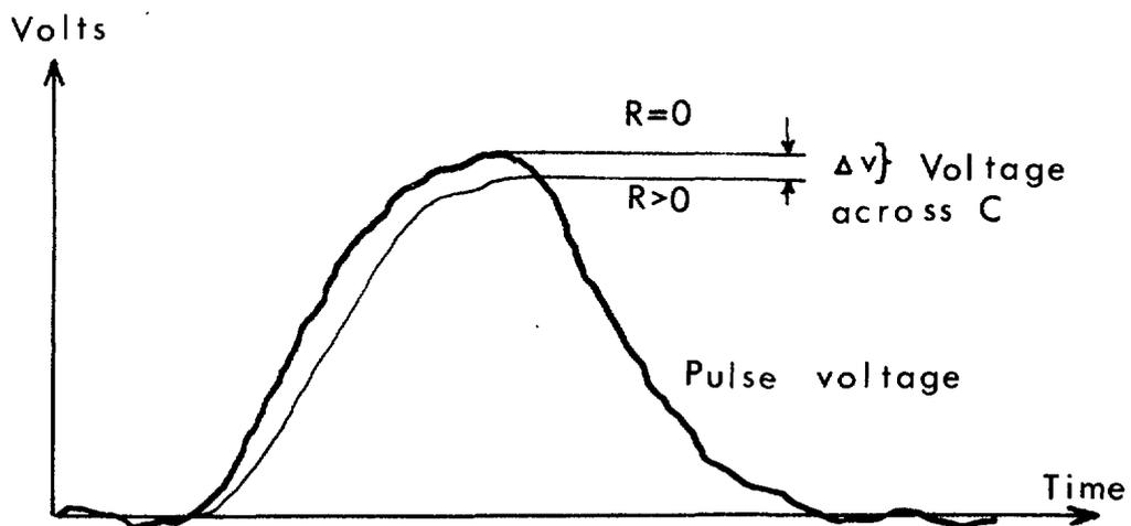
Fig. 2. The voltage across C for two different values of R,  $R = 0$  and  $R > 0$ .
