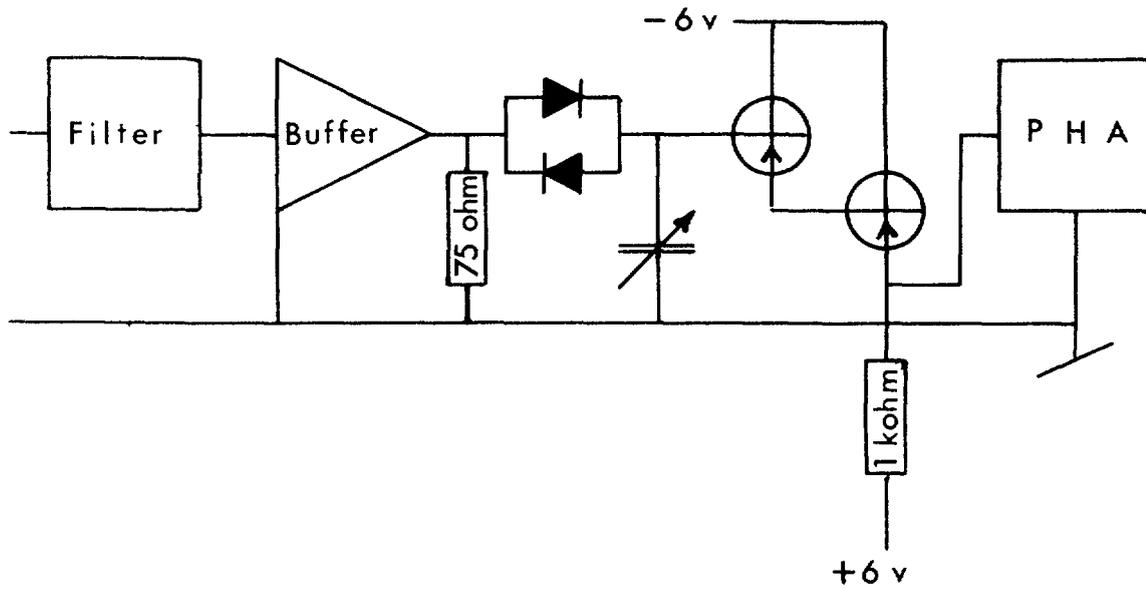
Fig. 3. The circuit between the buffer and the PHA is used to optimize the performance of the pulse height analyzer. Germanium diodes and silicon transistors have been used.
