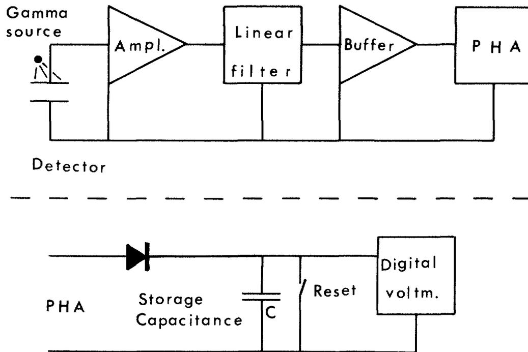
Fig. 1. Principle of pulse height measurement and of P H A = pulse height analyzer.
