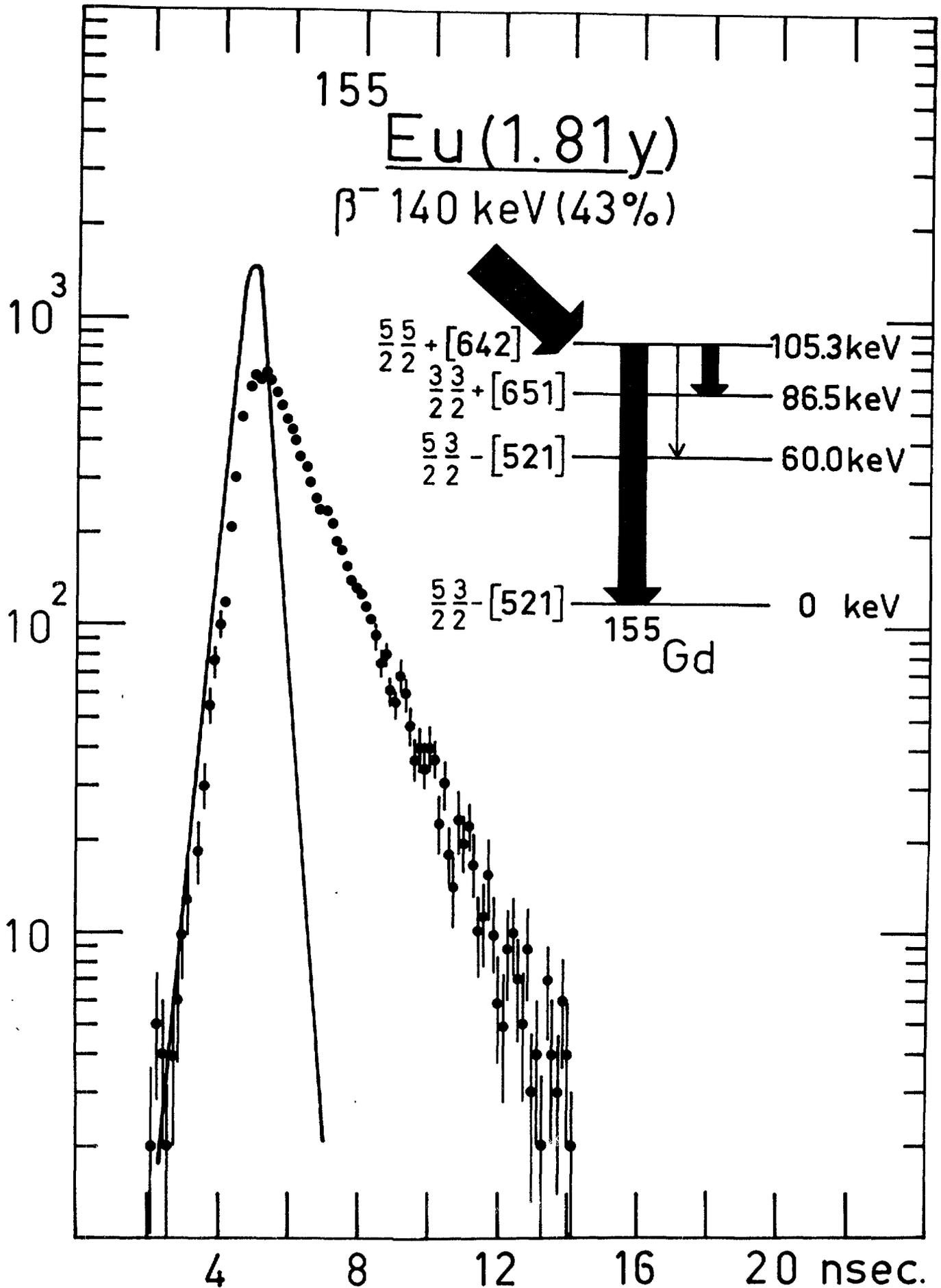
Fig. 2 Delayed coincidence curve taken between the 105.4 L electron line and the  $\beta^-$ -continuum at 135 keV giving  $T_{1/2} = 1.12 \pm 0.05$  nsec for the 105.4 keV level in  $^{155}\text{Gd}$ . The simplified decay scheme shows the principal feeding and deexcitation of the 105.4 keV level.
