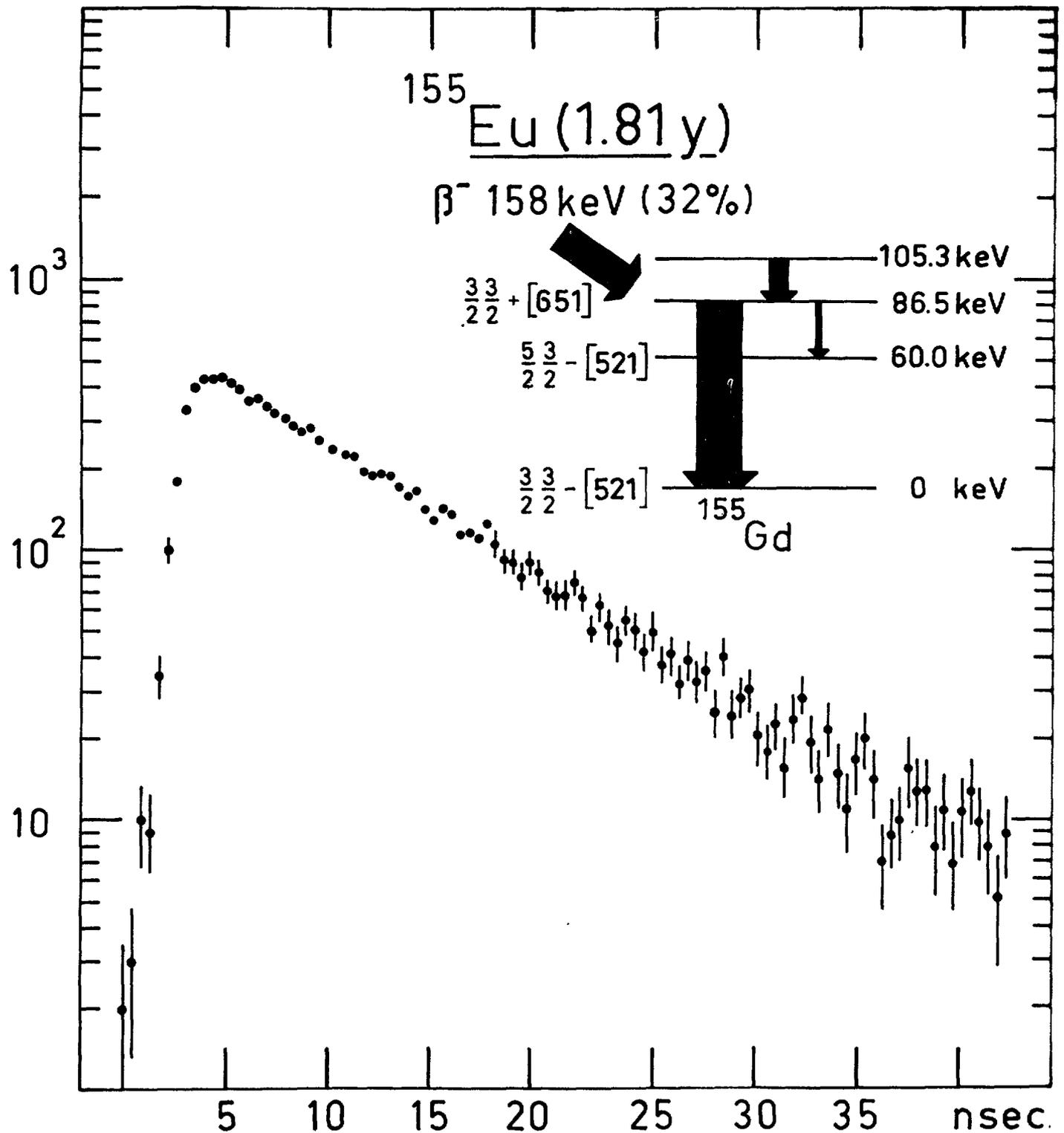
Fig. 1 Delayed coincidence curve taken between the 86.5 K electron line and the  $\beta^-$ -continuum at 135 keV giving  $T_{1/2} = 6.48 \pm 0.26$  nsec for the 86.5 keV level in  $^{155}\text{Gd}$ . The simplified decay scheme shows the principal feeding and deexcitation of the 86.5 keV level.
